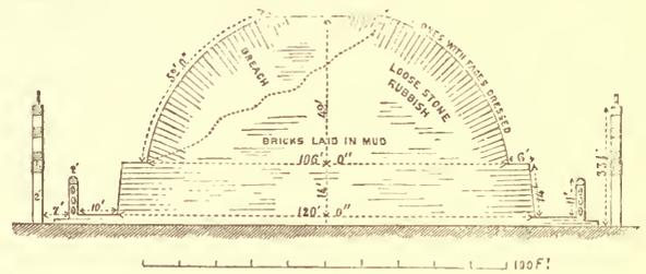
FIG. 25.—Section of Tope at Sanchi.
