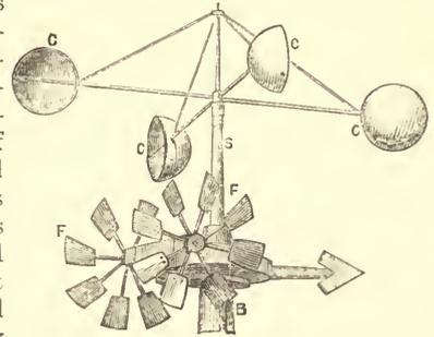
FIG. 1.—Cups and Vane of Anemometer.
