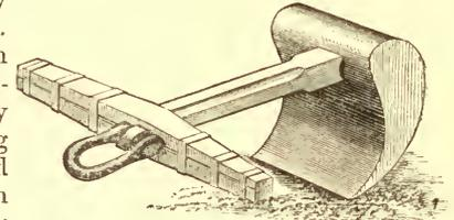
FIG. 10.—Cast-iron Mooring Anchor.
