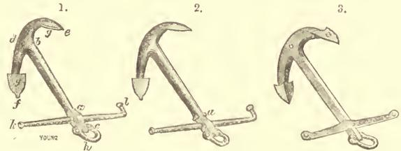
FIG. 1.—Common Anchor. FIG. 2.—Admiralty's. FIG. 3.—Rodger's.
