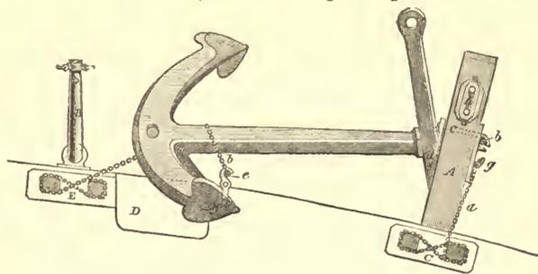
FIG. 7.—Bower Anchor, and manner of stowing.
