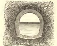
FIG. 2.—Tunnel in soft ground.
