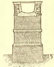
FIG. 17.—Section through Pier.
