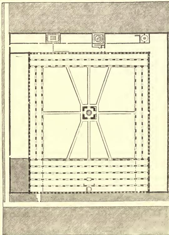
FIG. 46.—Plan of Mosque of Tooloon, Cairo. From Coste's *Architecture Arabe en Caire*.
