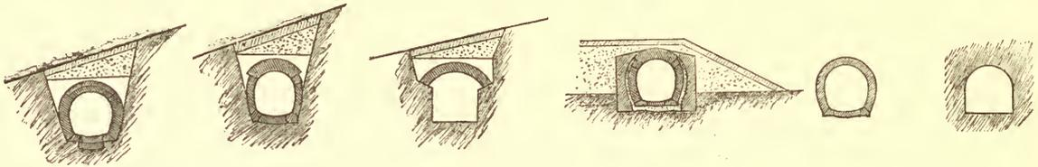
FIG. 6.—Open cutting not water-tight. FIG. 7.—Open cutting water-tight, but lined. FIG. 8.—Open cutting in rock. FIG. 9.—Aqueduct above surface of ground. FIG. 10.—Tunnel lined. FIG. 11.—Tunnel through water-tight rock.
