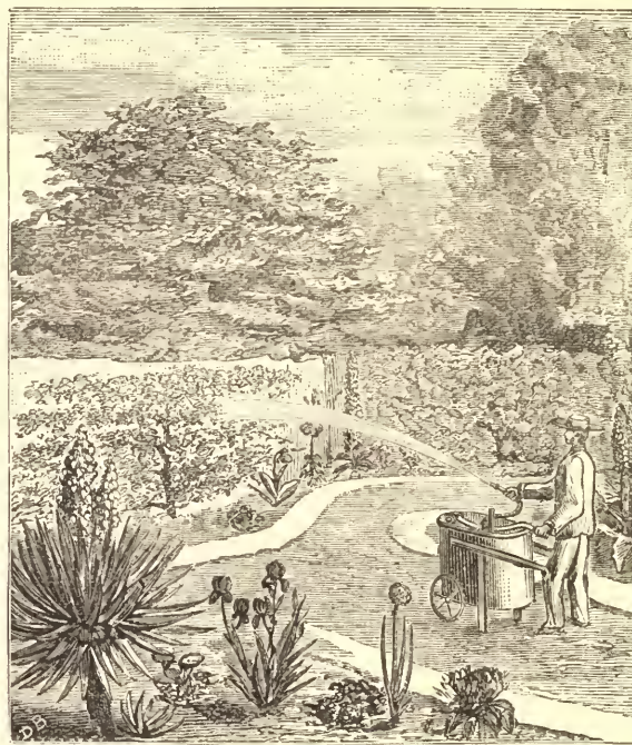
FIG. 50.—Read's Garden Engine.
