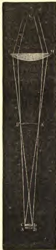
FIG. 3.—Diagram of Simplest Form of Compound Microscope.
