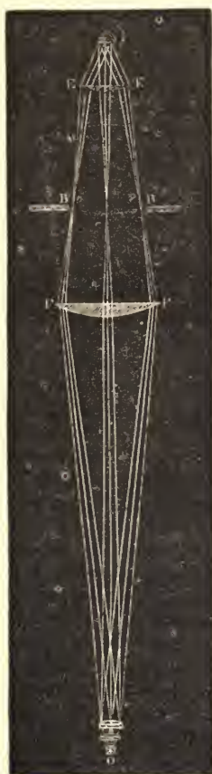
FIG. 4.—Diagram of Complete Compound Microscope.
