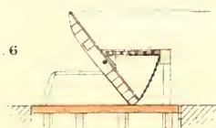
SELF ACTING WEIR ON RIVER IRWELL
