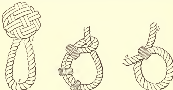
Fig. 19.—Sprit-Sail Sheet Knot. Fig. 20.—Turning in a Dead-Eye Cutter-Stay fashion. Fig. 21.—Turning in a Dead-Eye end up.
