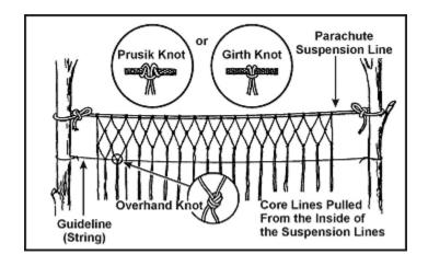
Figure 8-20. Making a Gill Net
