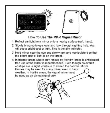
Figure 19-3. MK-3 Signal Mirror
