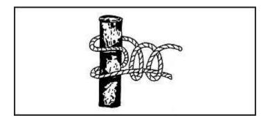
Figure G-4. Round Turn and Two Half-Hitches
