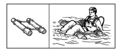
Figure 17-8. Log Flotation
