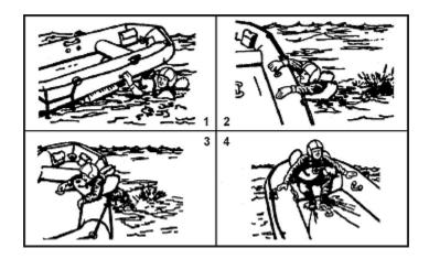
Figure 16-14. Method of Boarding Seven-Man Raft
