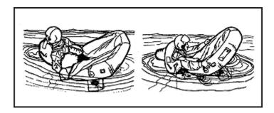
Figure 16-10. Other Methods of Boarding the One-Man Raft
