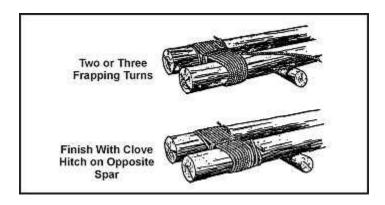
Figure G-14. Shears Lashing
