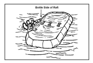
Figure 16-13. Method of Righting Raft
