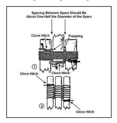
Figure G-16. Tripod Lashing
