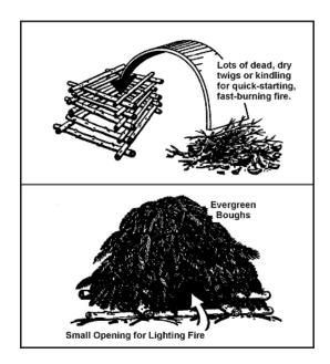
Figure 19-2. Smoke Generator—Ground
