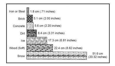
Figure 23-1. Materials to Reduce Gamma Radiation
