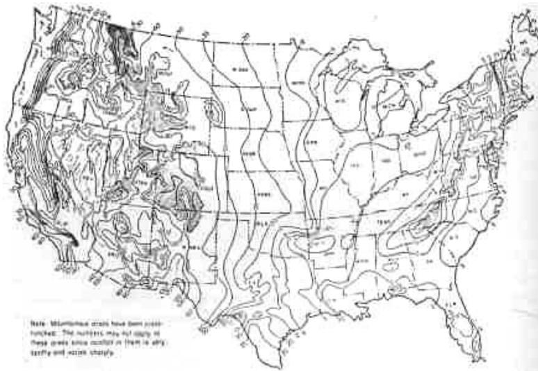
Approximate acreage required in the drainage area for each acre-foot of water stored in an embankment or excavated pond.
