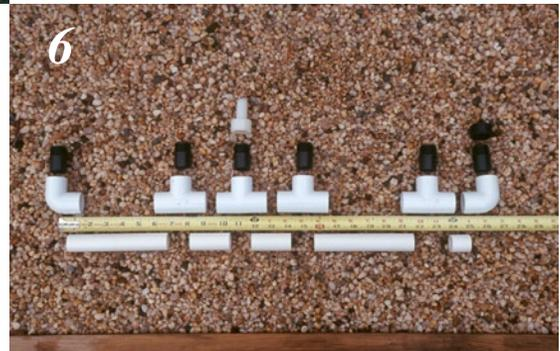
**Step 7.** Assemble the internal spray lines from the parts shown here - 3/4" FGH swivel adapter with a compression end, .375 ID poly spray line, 10 mm insert plug and a 1" rubber grommet to seal the entry point of the spray line into the growth chamber.
