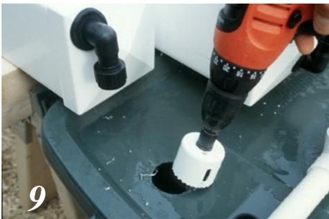
**Step 9.** Using a 1.5" hole saw, cut a hole for each chamber's drain fitting to mate with the lid of your reservoir. I have found the simplest way to measure and mark off the location for these holes is to connect all chambers to the injection manifold, position them over the reservoir and mark the center of each drain hole by sighting down each drain fitting.
