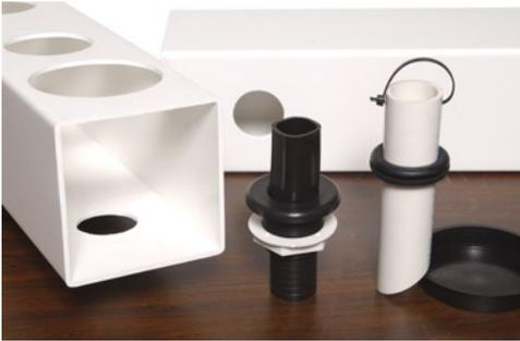
**Note.** There are actually two options available when making the drain stems. The first would be to use the bulkhead fitting and nut as shown at left, the second is to use a rubber grommet and 1 1/4" PVC stub. Cost and availability of the materials will help you decide as I've found both to work equally as well.
