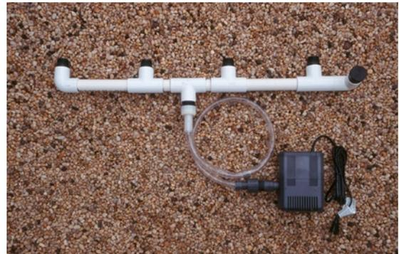
*Note. Once you insert the spray lines into the compression end of the adapters, they are nearly impossible to remove without damage. Test fit everything first! You only need to insert about 1/2" into the compression end for a good seal.*
