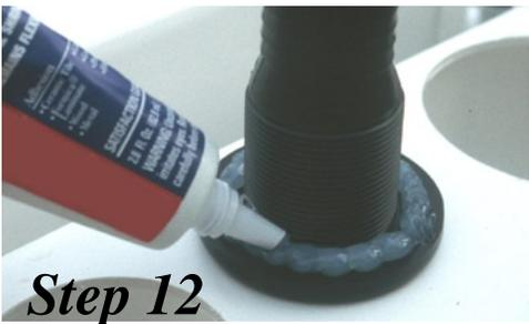
**Step 12.** If you choose to use the bulkhead fitting, be sure to seal with Aquarium-safe silicone sealant to prevent leaks. Apply as shown here. If you choose to go with the grommet method, it helps to apply a thin coating of nontoxic silicone grease to the inside of the grommet to allow the level tube to move up and down easily.
