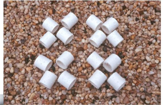
*Cut 3/4" - 1" sections of 1/2" PVC pipe to make the spray line clips shown above. They are glued into the chambers using PVC cement. For best results, use PVC primer before applying glue to soften the material and provide a better glue joint.*
