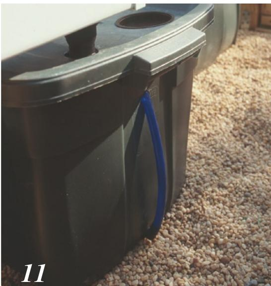
**Step 11.** A 7/8" hole in the bottom of the reservoir wall accepts a 1/2" ID rubber grommet, 1/2" barbed elbow and 1/2" blue level tubing to complete your nutrient reservoir level indicator
