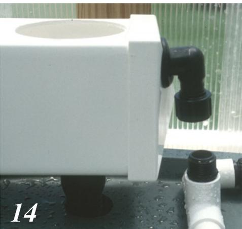
**Step 14.** You are now ready to connect the chambers to the injection manifold as shown in the sequence of photos here.
