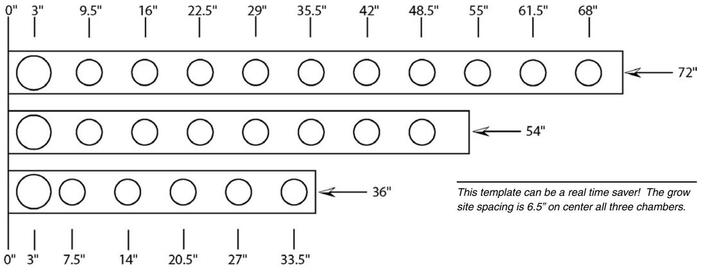
*This template can be a real time saver! The grow site spacing is 6.5" on center all three chambers.*
