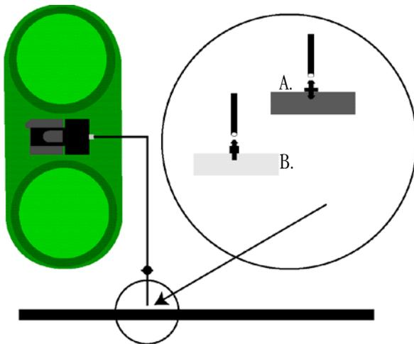
A. Rigid PVC pipe use 10/32" threaded joiners with teflon tape
