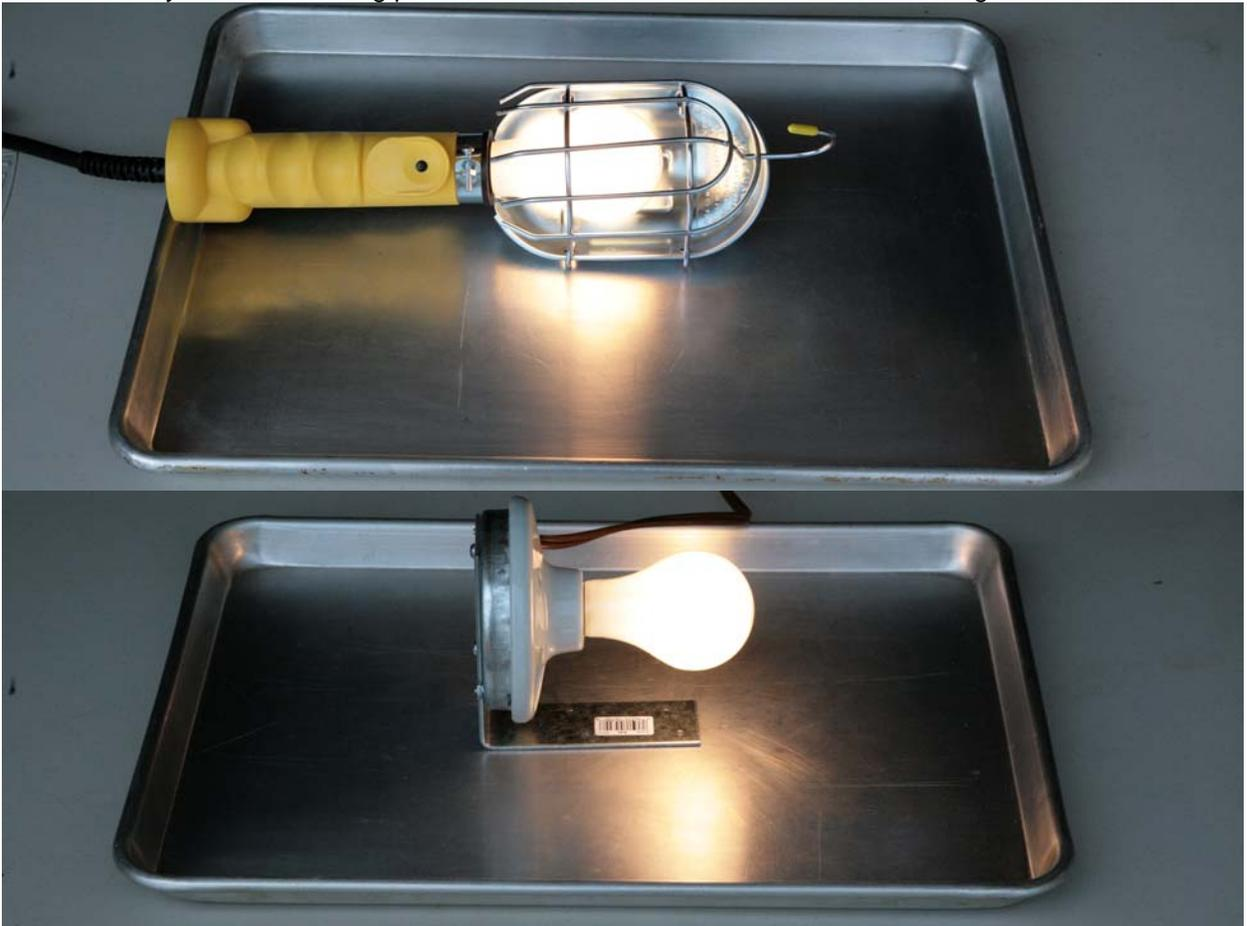
11. Place your box assembly over the heat source which should be centered in the bottom of the box.
