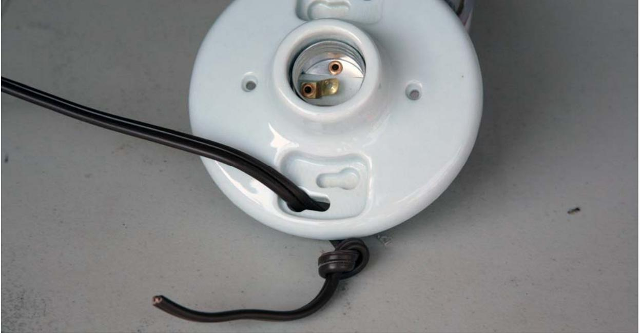
6. Unzip the two wires of the cord back to the knot. Strip about 1" of insulation from each of the wires and twist the ends of the wires tightly to keep the strands of small wire from unraveling.
