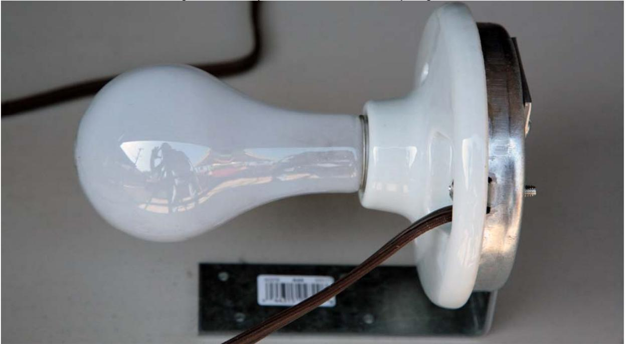
12. As an option, if the long screws used to mount the lamp holder to the electrical box protrude beyond the back of the electrical box, you can put 8-32 nuts on them to give a more finished look. This completes the heater assembly.
