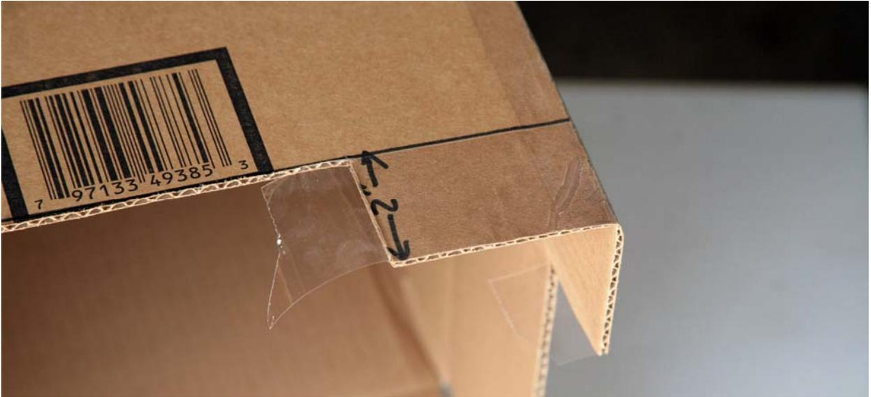
7. Fold the loose ends of the tape over the edges and press to the back side of the 3" legs. This will reinforce the corners so that it will support a significant amount of weight. Repeat step 6 and 7 until all 4 corners have been reinforced.
