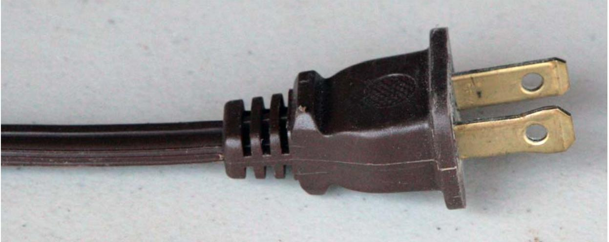
8. Now secure the wire that is on the same side as the wide blade of the plug under the silver screw on the bottom of the lamp holder. Then secure the wire that is on the same side as the narrow blade of the plug under the gold screw on the bottom of the lamp holder. Don't worry, if you mix the wires up the lamp will still work just fine. The rather fiddly step of identifying the different wires just assures that the wires are connected as suggested by the National Electrical Code.
