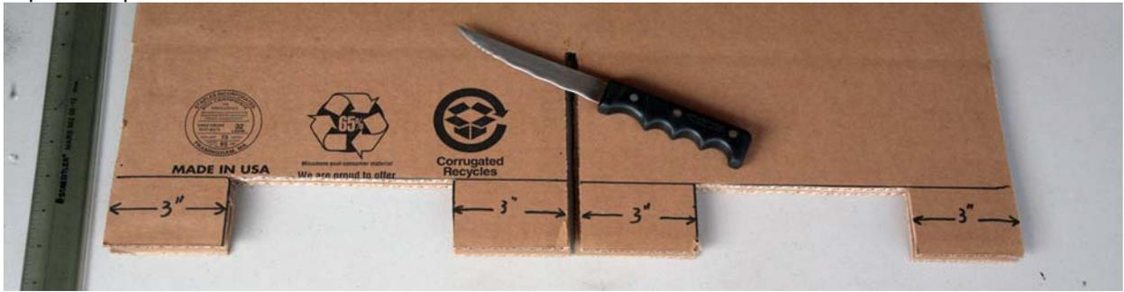
4. Move to the top set of flaps. Draw a line 2" below the point where the flaps fold. Turn the box over and do the same on the other side.
