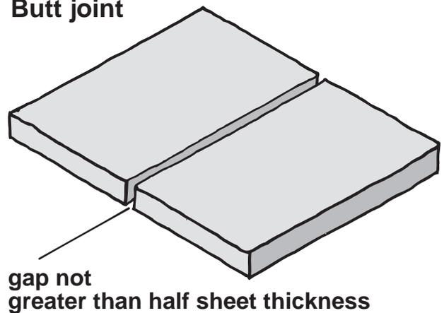
The gap between the edges depends on the joint type and sheet thickness.
