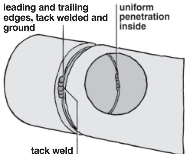
Root runs can be made by TIG or MIG/MAG with dip or pulse techniques or by MMA welding. With TIG welding the bore of the pipe can be filled with argon or nitrogen to protect the penetration bead and to control its profile.
