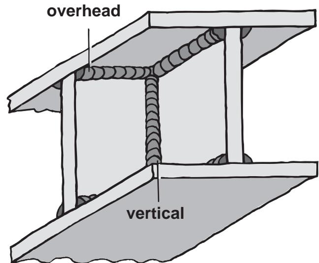
The appropriate technique for these types of joint is either ‘Dip Transfer’ or ‘Pulse Transfer’.
