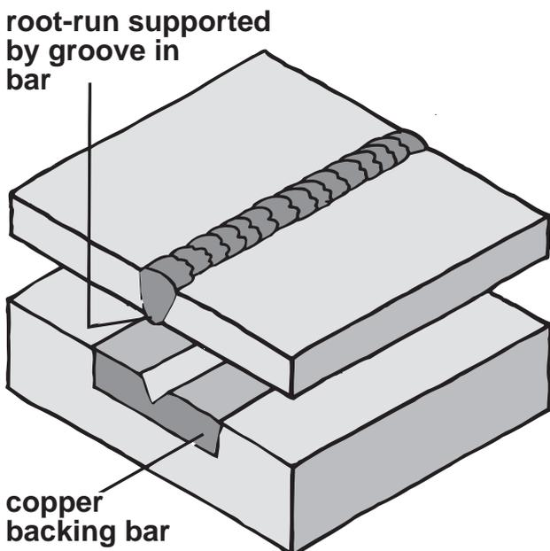
Alternatively, the underside of the root run can be supported by a backing bar which is removed after welding or a backing strip which is left in place.
