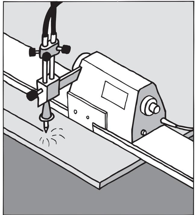
Mechanised systems can be used to prepare the edges of plate prior to welding.
