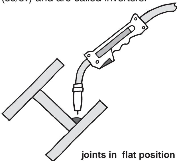
The process can be operated at currents within the range 280–500A for welding plates, thick walled pipes and sections in the flat position. The term ‘Spray Transfer’ is used to describe this type of operation.
