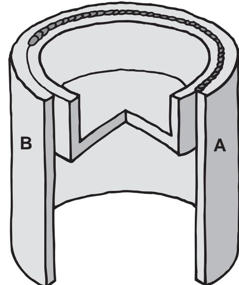
conventional TIG - welding speed progressively increased from A-B
