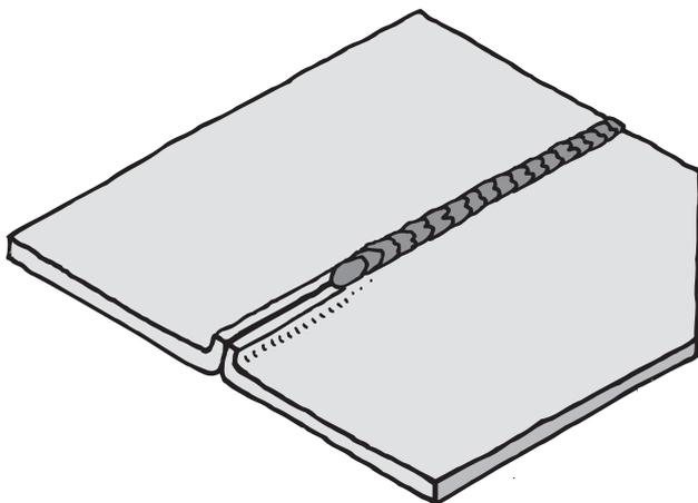
Butt joints in sheet less than 1mm thick are TIG welded. The edges of the sheet can be flanged to avoid the need to use filler metal.
