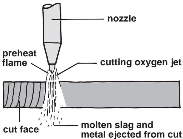
The cutting action depends on a chemical reaction between oxygen and hot iron or steel.
