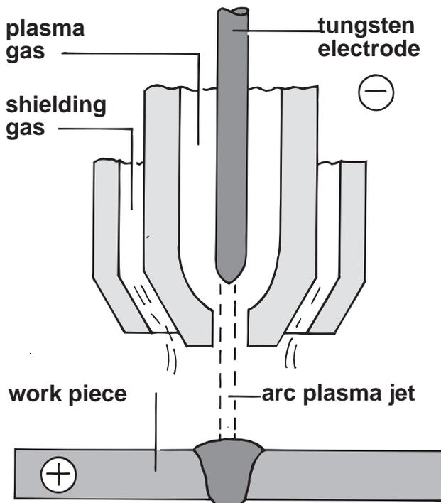
Plasma arc welding relies on a special technique known as keyholing. First a hole is pierced through the joint by the plasma arc. As the torch is moved along the joint, metal melts at the front of the hole, swirls to the back and solidifies.
