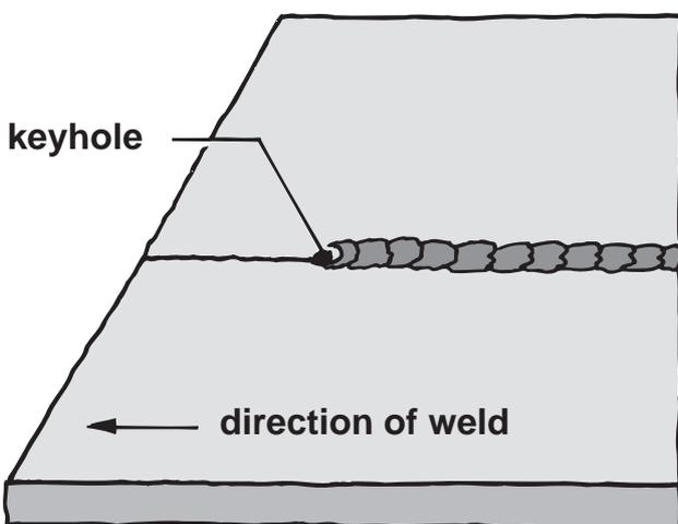
Plasma arc welding is mainly used for butt joints in plates and pipes. Its principal advantage is that it gives controlled penetration.
