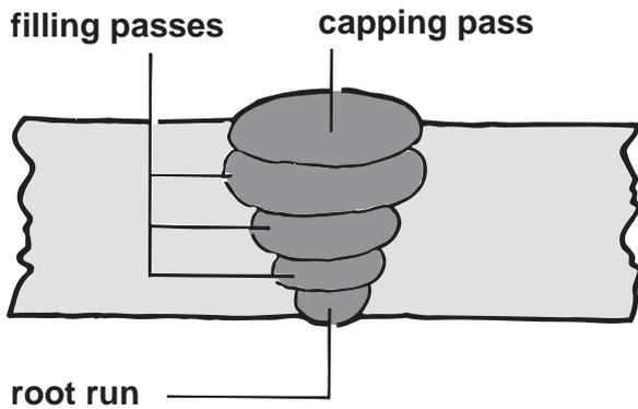
The deep penetration characteristic of spray transfer makes it difficult to control the molten metal in a root run. The root run can be deposited with dip, or MMA welding can be used.
