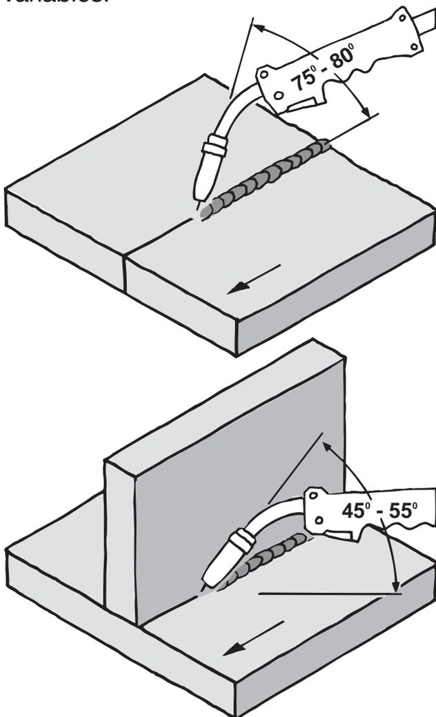
**Voltage** controls the profile of the weld. **Inductance** (in Dip Transfer) stabilises the arc and minimises spatter. **Wire feed speed** sets the welding current.
