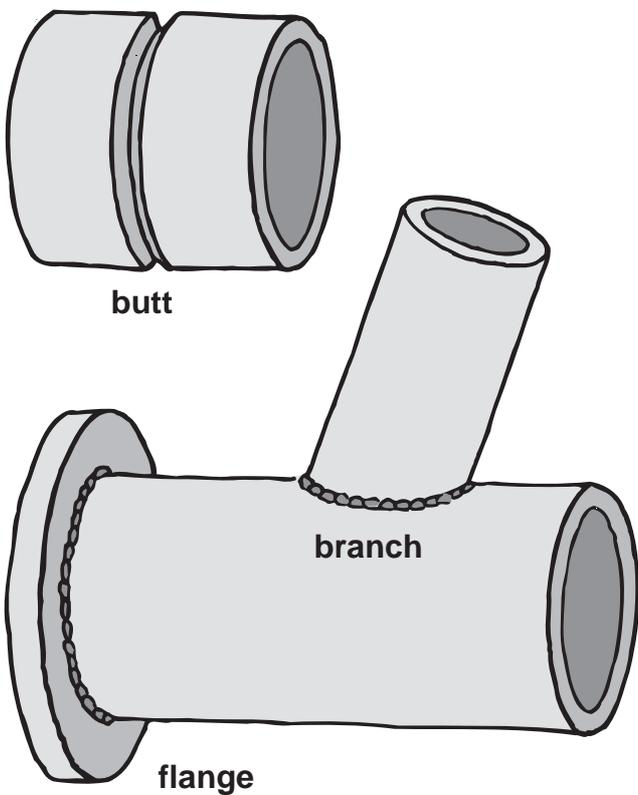
If possible, during welding the pipe should be *rotated* so that the weld is made in the horizontal position - use spray, dip or pulse transfer for MIG/MAG.
