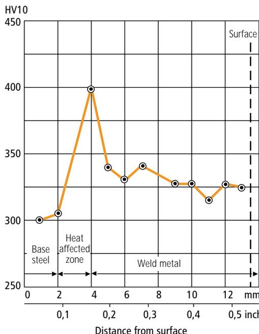
Note the uniform hardness distribution, only marginally higher than the base hardness, and the very narrow heat-affected zone with only a modest hardness increase at the fusion line.
