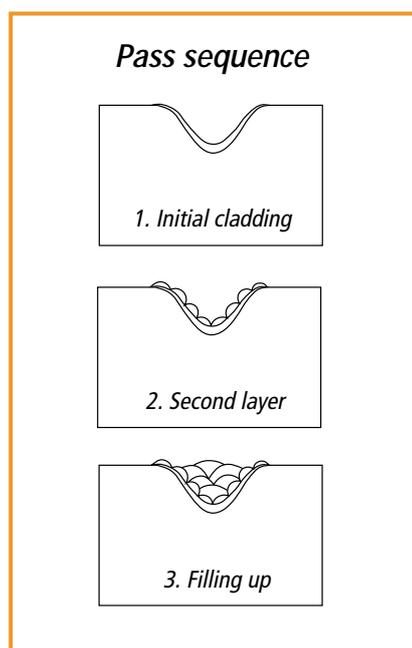
If copper or graphite support is used, an extra 1,5 mm (0,06 inch) must be allowed between the support and the required weld surface because the slag takes up a certain amount of space (MMA welding).
