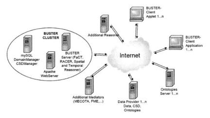
Fig. 7.1. BUSTER: system architecture.
