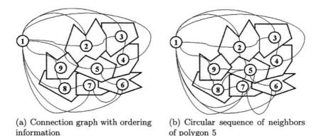
Fig. 5.7. Connection graph representation of a decomposition by tessellation.
