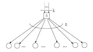
Fig. 4.1 A network representation of a classical linear block code.
