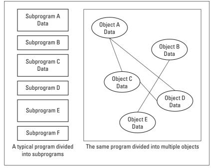
Figure 19-3: In objectoriented programs, objects isolate data from other objects.
