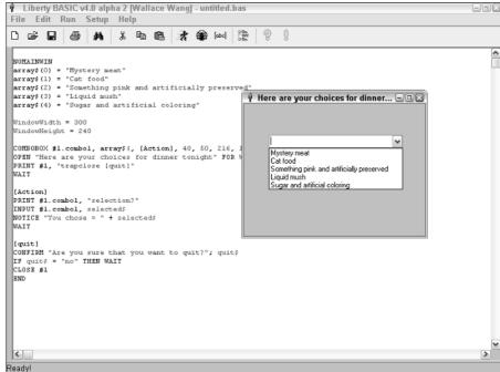
Figure 14-8: Combo boxes display a dropdown list.
