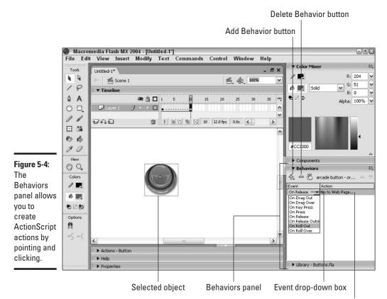
Double-clicking an action allows you to input parameter values for that action
