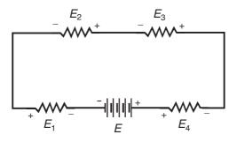
**Figure DC13-1** According to Kirchhoff's voltage law, the sum of the voltages across the resistances in a series DC circuit is equal and opposite to the battery voltage. If we disregard polarity, then in this example, we'll observe that  $E = E_1 + E_2 + E_3 + E_4$ .
