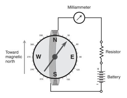
**Figure DC22-3** Arrangement for testing the galvanometer. Be sure that the compass needle points exactly toward N on the scale under no-current conditions, and deflects toward the east of N when current flows through the coil.
