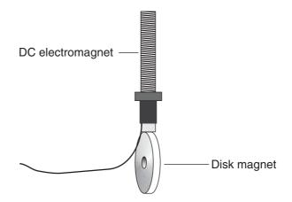
**Figure MRG10-2** *Disk magnet "hanging" from the end of an electromagnet's core when no current flows through the coil. What will happen when you connect the electromagnet's coil to a lantern battery?*
