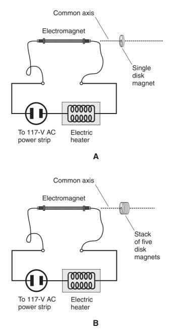
Figure MAG13-1 At A, a single disk magnet near an AC electromagnet. At B, a stack of five disk magnets near an AC electromagnet.
