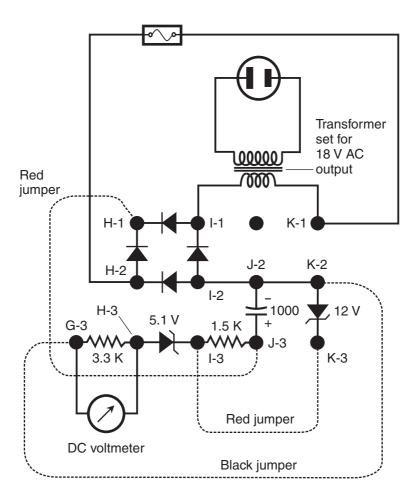
**Figure AC17-4** *Measurement of the voltage across a 3.3-K load with a 12-V Zener diode in parallel and a 5.1-V Zener diode in series.*
