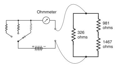
Figure DC11-1 Resistive network with 326 ohms across a series combination of 981 ohms and 1467 ohms.
