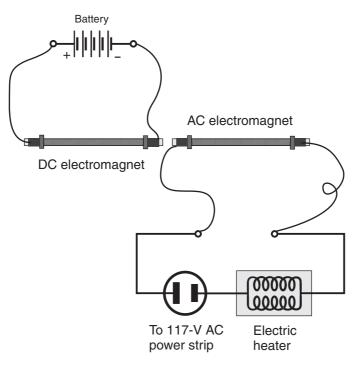
**Figure MAG14-1** An AC electromagnet placed end-to-end with a DC electromagnet.
