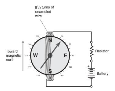
**Figure DC22-1** The galvanometer and associated circuitry. The compass must lie flat on a horizontal surface, and must be placed so the needle points toward N (magnetic azimuth  $0^{\circ}$ ) when the battery is disconnected.
