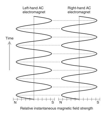
**Figure MRG15-2** Interaction of AC electromagnets as they repel. Each dashed line represents maximum repulsion between like poles in close proximity.
