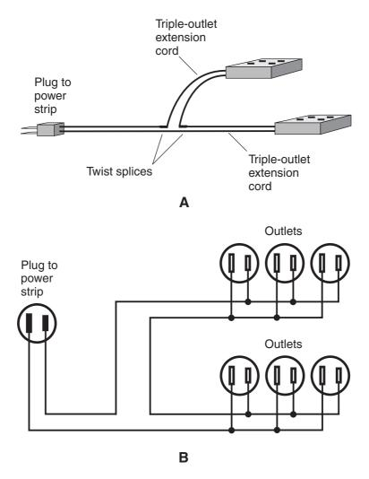
**Figure AC2-1** *Extension-cord interconnection to obtain two sets of outlets in series. At A, the pictorial diagram. The twist splices must be completed and insulated before the assembly is connected to any power source. At B, the schematic diagram.*
