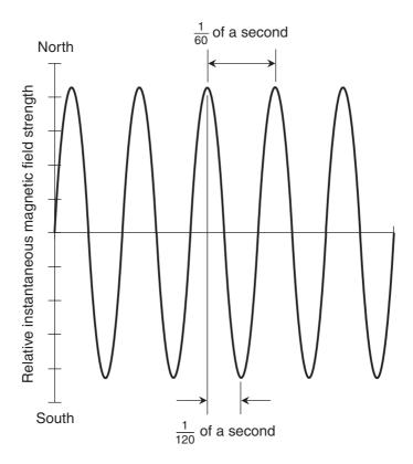
Figure MAG12-2 Instantaneous field strength as a function of time at one end of an AC electromagnet supplied with 117-V RMS at 60 Hz.
