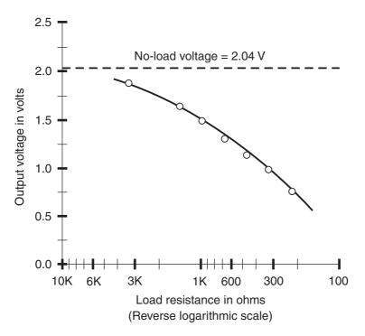
**Figure DCI4-5** *Output voltage versus load resistance for the resistive voltage divider. These are my results. The dashed line shows the open-circuit (no-load) voltage. Open circles show measured voltages under various loads. The solid curve approximates the circuit's characteristic function.*
