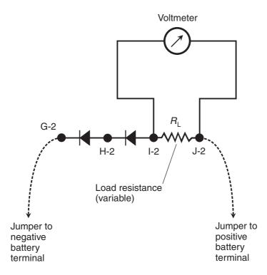
**Figure DC15-3** Suggested arrangement for measurements of the voltages across the load resistance in a two-diode voltage reducer. Solid dots show breadboard terminals. Dashed lines indicate jumpers. Pay attention to the diode polarity! The cathodes should go toward the negative battery terminal.
