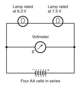
Figure DC19-2 Measurement of voltage *E* across the combination of two dissimilar lamps in series.
