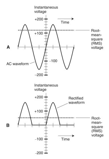
**Figure AC4-2** Half-wave rectification. At A, the AC waveform as it appears at the power strip. At B, the output waveform as it appears at the cord outlets and across the lamp. Dashed lines indicate root-mean-square (RMS) or effective voltages.
