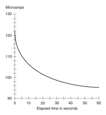
**Figure DC5-1** Graph of maximum deliverable current as a function of time from my "body cell." My hands were wetted with a solution of three rounded teaspoons of salt dissolved in 12 fluid ounces (fl oz) of vinegar.
