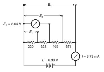
**Figure DC14-3** Network for testing the operation of a resistive voltage divider. All resistance values are in ohms. The battery voltage *E*, the voltage across the first and second resistors, and the resistances are those I measured.
