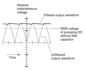
**Figure ACI4-1** A filter capacitor "smooths" the output of a full-wave rectifier by charging with each pulse, holding the voltage near the peak value.
