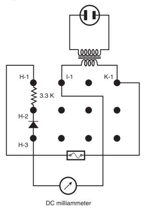
**Figure AC7-4** *Measurement of the pulsating current that the transformer-diode combination drives through a resistive load.*
