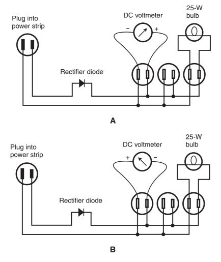
**Figure AC4-3** At A, measurement of the effective DC voltage with the meter polarity matching the rectifier output polarity. The meter shows a positive value. At B, measurement of the effective DC voltage with the meter polarity reversed. The meter displays a negative value, but the absolute voltage is the same as before.
