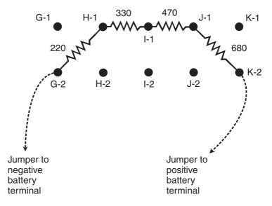
Figure DC13-2 Suggested arrangement of resistors on breadboard for demonstration of Kirchhoff's voltage law. All resistance values are in ohms. Solid dots indicate terminals. Dashed lines indicate jumpers.
