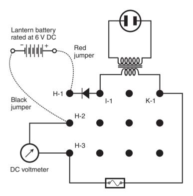
**Figure AC9-3** *Measurement of the open-circuit pulsating DC output voltage from the transformer-diode-battery combination with the battery connected "backward" so its voltage subtracts from the rectified voltage.*
