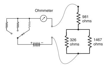
**Figure DC11-5** *Resistive network with 981 ohms in series with a parallel combination of 326 ohms and 1467 ohms.*
