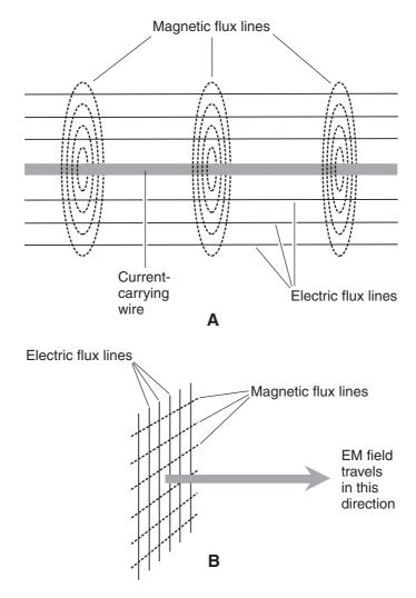
**Figure AC18-1** At A, the electric and magnetic lines of flux around a straight, current-carrying wire. At B, the flux lines far from a current-carrying wire. The EM field travels straight away from the wire, in a direction perpendicular to both sets of flux lines.
