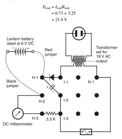
**Figure AC12-3** *Measurement of the filtered output current through a load from the power supply and battery in series, with the battery bucking the supply.*
