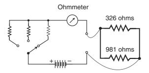
**Figure DC10-1** *Parallel combination of 326-ohm and 981-ohm resistances.*
