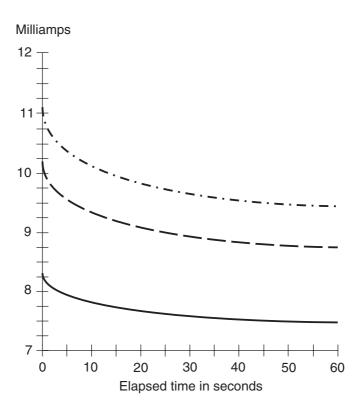
**Figure DC4-3** Graphs of maximum deliverable currents as functions of time for various amounts of salt dissolved in 12 fluid oz (0.36 L) of vinegar. Lower (solid) curve: one rounded teaspoon of salt. Middle (dashed) curve: two rounded teaspoons of salt. Upper (dashed-and-dotted) curve: three rounded teaspoons of salt.
