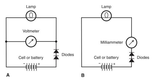
**Figure DC16-2** At A, the arrangement for measuring the voltage across a lamp with diodes in series. At B, the arrangement for measuring the current through a lamp with diodes in series. Pay attention to the diode polarity!
