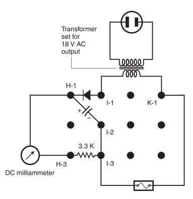
**Figure AC12-1** *Measurement of the filtered output current through a load from the power supply alone.*
