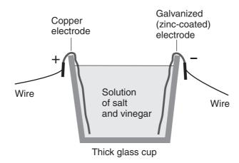
**Figure DC4-2** A wet cell made from a vinegar-andsalt solution. The glass cup has a brimful capacity of approximately 12 fluid oz (0.36 L).
