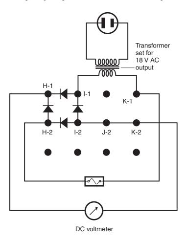
**Figure AC13-2** *Measurement of the open-circuit pulsating DC output voltage from the bridge rectifier circuit.*
