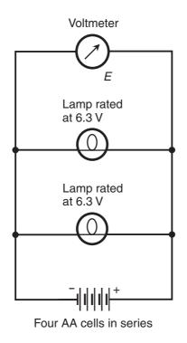
Figure DC20-3 Measurement of voltage E across the combination of two "identical" lamps in parallel.
