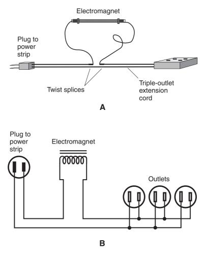
**Figure MAG12-1** Extension-cord modification to connect electromagnet in series with AC outlet. Twist and insulate the splices (drawing A) before you connect the assembly to the power source. Illustration B shows a schematic of the complete system.
