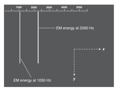
**Figure AC18-2** The DigiPan display system. The horizontal or x axis portrays frequency. The vertical or y axis portrays time. The EM-field "signals" show up as steadily lengthening vertical lines. This drawing shows two hypothetical examples.
