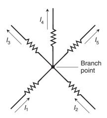
**Figure DC12-2** According to Kirchhoff's current law, the sum of the currents flowing into any branch point is equal to the sum of the currents flowing out of that branch point. In this example,  $I_1 + I_2 = I_3 + I_4 + I_5$ .
