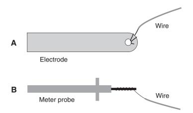
**Figure DC4-1** Attachment of wires to the electrodes (at A) and the meter probes (at B). Wrap the bare wire around the metal. Then secure the connections with electrical tape.
