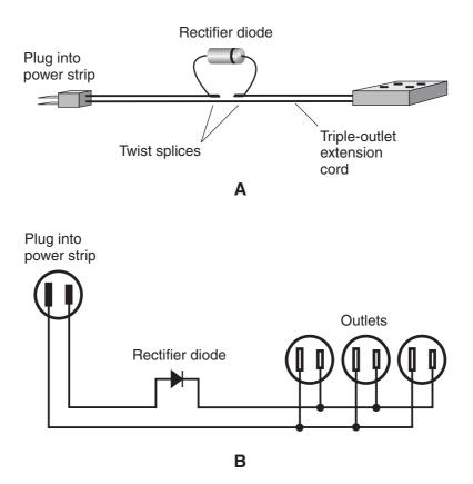
**Figure AC4-1** Drawing A is a pictorial diagram showing the construction of the rectifier cord. The twist splices must be completed, and insulated with electrical tape, before the assembly is connected to any source of power. Drawing B is the schematic circuit diagram.
