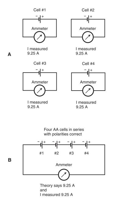
**Figure DC3-1** *I* short-circuited four different AA cells with an ammeter, and estimated that each cell produced 9.25 A as shown at A. Then I connected the cells in series so that they all worked together, shorted the combination with the ammeter, and got 9.25 A again as shown at B.
