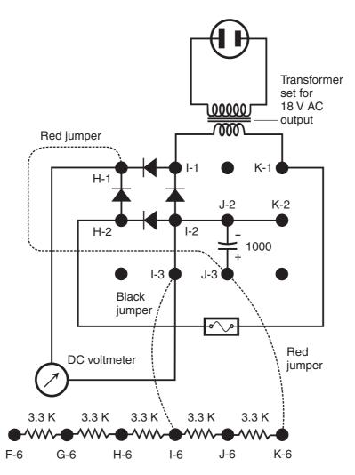
**Figure AC15-2** *Testing the behavior of a filter capacitor after removal of power with a bleeder resistance to speed up the discharge process.*
