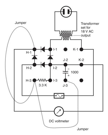
**Figure AC14-3** *Measurement of the DC voltage from the filtered full-wave bridge power supply across a resistive load.*
