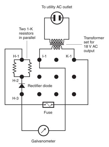
**Figure AC6-1** Suggested breadboard arrangement for testing a galvanometer with diode-rectified AC. The resistors should be rated at 1/2 W, and the transformer should be set for 18 V output. Black dots represent breadboard terminals.
