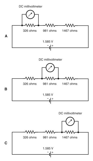
**Figure DC8-2** Schematic diagrams of the arrangements I used to measure the voltage produced by a current of 553  $\mu$ A through a 326-ohm resistance (A), a 981-ohm resistance (B), and a 1467-ohm resistance (C).
