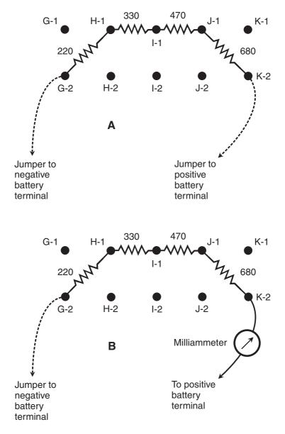
Figure DCI4-2 At A, suggested arrangement for measurements of the voltages across individual resistors. All resistance values are in ohms. Solid dots indicate terminals. Dashed lines indicate jumpers. At B, suggested arrangement for measurement of current through the network.
