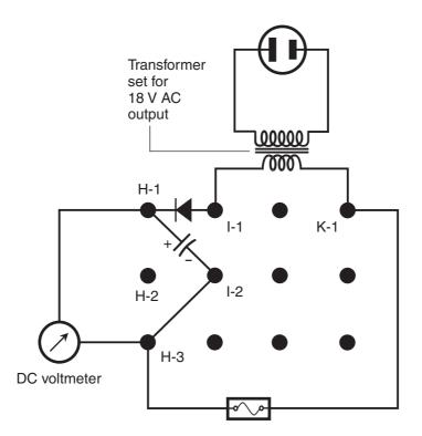
**Figure ACID-1** Measurement of the open-circuit filtered DC output voltage from the transformer-diode-capacitor combination alone. This is the same circuit that you built according to Fig. AC8-1, but the components are arranged differently to accommodate future tests.
