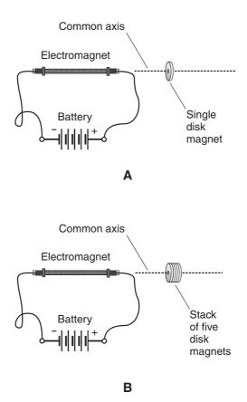
**Figure MAG10-1** At A, a single disk magnet near a DC electromagnet. At B, a stack of five disk magnets near a DC electromagnet.
