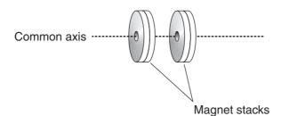
Figure MRG 4-1 When you bring two permanent magnets near each other and place them along a common axis, you can feel the magnetic force between them.
