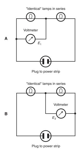
**Figure AC2-2** At A, measurement of voltage  $E_1$  across the bulb in the left-hand of two "identical" lamps in series (called L). At B, measurement of voltage  $E_2$  across the bulb in the right-hand lamp (called R).
