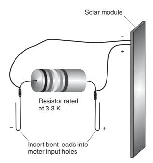
**Figure DC25-2** Arrangement for installing the solar module and parallel resistor. Be sure that the solar module polarity matches the meter polarity.
