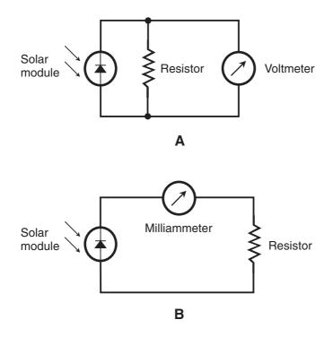
Figure DC24-1 At A, the circuit for measuring solar-module output voltage versus load resistance. At B, the circuit for measuring solar-module output current versus load resistance.
