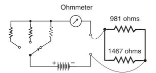
**Figure DC10-3** *Parallel combination of 981-ohm and 1467-ohm resistances.*
