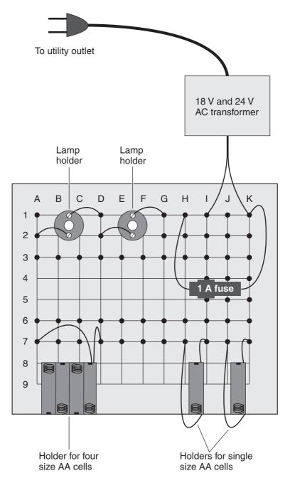
**Figure AC5-1** Breadboard arrangement for wiring the AC transformer and fuse. The low-voltage, fused AC output appears between terminals H-1 and I-1.
