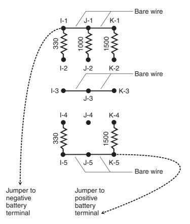
Figure DC12-1 Arrangement of resistors on breadboard for demonstration of Kirchhoff's current law. All resistance values are in ohms. Solid dots indicate breadboard terminals. Solid lines show interconnections with bare copper wire. Dashed lines indicate jumpers.
