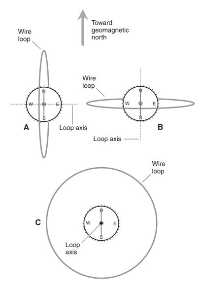
Figure MAG8-3 Relative positions of wire loop and compass. At A, loop axis running east-west with compass at center. At B, loop axis running north-south with compass at center. At C, loop axis oriented vertically with compass at center. (All views are looking straight down at the compass.)
