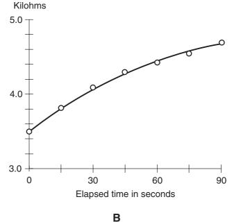
**Figure DC7-1** At A, the arrangement for measuring the resistance of tap water. At B, the resistance values as I measured them over a time span of 90 seconds.
