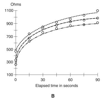
Figure DC7-3 At A, the arrangement for measuring the resistance of water with soda (sodium bicarbonate) fully dissolved. At B, the resistances I observed over a span of 90 seconds. Upper (short-dashed) curve: 0.5 teaspoon of soda. Middle (long-dashed) curve: 1.0 teaspoon of soda. Lower (dashed-and-dotted) curve: 1.5 teaspoons of soda.
