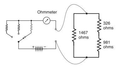
Figure DC11-3 Resistive network with 1467 ohms across a series combination of 326 ohms and 981 ohms.
