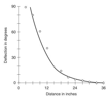
**Figure MRG 3-3** *Graph of the eastward compass deflection versus the distance from a stack of five disk magnets. Open circles show measured values; the solid curve approximates the function.*
