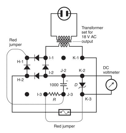
**Figure AC16-1** Addition of a current-limiting resistance R and a Zener diode D to regulate the DC output voltage from a filtered full-wave rectifier. The meter is connected to measure the regulated output voltage under no-load conditions.
