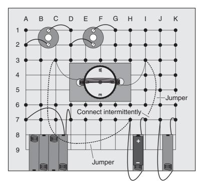
**Figure DC22-2** Suggested placement of the galvanometer on the breadboard. The jumper for the positive cell terminal is normally disconnected. This jumper should never be connected to the cell for more than a couple of seconds at a time.
