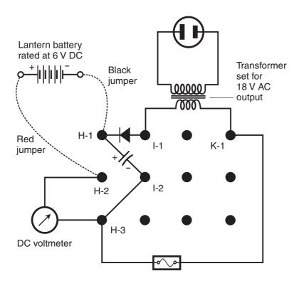
**Figure ACID-2** Measurement of the open-circuit filtered DC output voltage from the transformer-diode-capacitor-battery combination with the battery connected "forward" so its voltage adds to the power-supply voltage.
