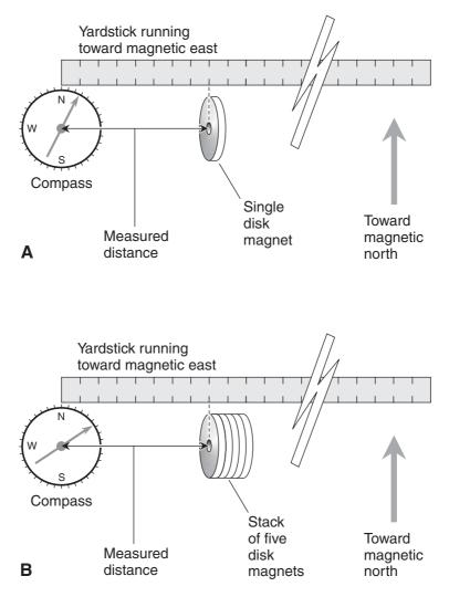
**Figure MRG 3-1** At A, the arrangement for testing the effect of a single disk magnet on a compass. At B, the arrangement for testing the effect of a stack of five disk magnets. Distances should be measured between the center of the compass and center of the nearest magnet face.
