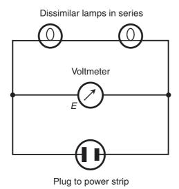
Figure AC3-2 Measurement of voltage E across the combination of two dissimilar
