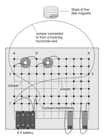
**Figure MRG6-2** Arrangement for reversing the direction of the current through the wires.
