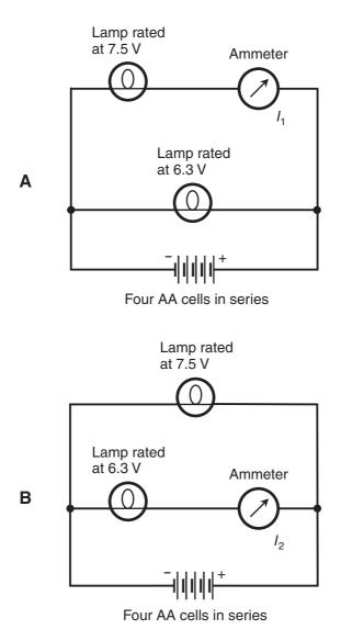
**Figure DC21-1** At A, measurement of current  $I_1$  through the "farther-from-battery" of two dissimilar lamps in parallel (called F, rated at 7.5 V). At B, measurement of current  $I_2$  through the "closer-to-battery" lamp (called C, rated at 6.3 V).
