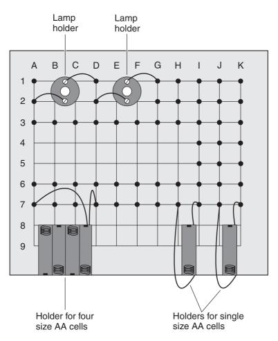
**Figure DC1-1** Layout of the breadboard for DC experiments. I used a "12-in" pine board (actually 10.8 in wide) with a thickness " $3/_4$  in" (actually about 0.6 in), cut to a length of 12.5 in. Solid dots show the positions of the nails. Grid squares measure 1 in by 1 in.
