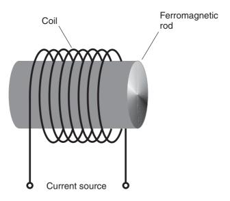
Figure MRG9-1 A simple electromagnet consists of a wire coil surrounding a rod made of ferromagnetic material.
