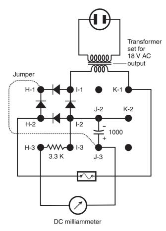
**Figure ACI4-4** *Measurement of the current that the filtered full-wave bridge power supply drives through a resistive load.*
