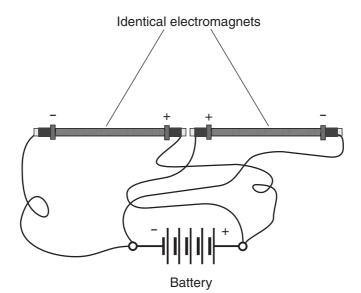
**Figure MRG11-2** *Electromagnets placed end-to-end with like poles in proximity.*
