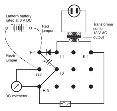
**Figure ACID-3** Measurement of the open-circuit filtered DC output voltage from the transformer-diode-capacitor-battery combination with the battery connected "backward" so its voltage subtracts from the power-supply voltage.
