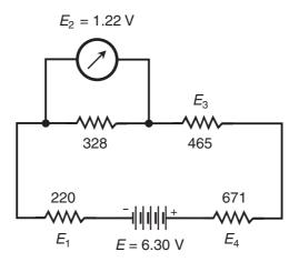
Figure DC13-3 Network for verifying Kirchhoff's voltage law. All resistance values are in ohms. The battery voltage E, the voltage across the second resistor, and the resistances are the values I measured.
