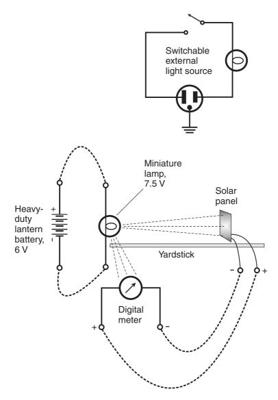
**Figure DC23-1** Arrangement for measuring solar-module output versus distance from miniature lamp. Dashed lines indicate jumper wires.
