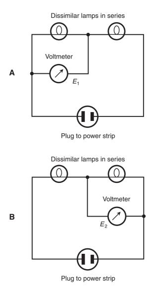
**Figure AC3-1** At A, measurement of voltage  $E_1$  across the bulb in the left-hand of two dissimilar lamps in series (called L). At B, measurement of voltage  $E_2$  across the bulb in the right-hand lamp (called R).
