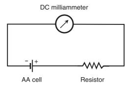
**Figure DC8-1** To measure the current that a known voltage drives through a known resistance, simply connect the voltage source, the resistor, and the meter in series.
