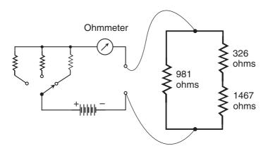
Figure DC11-2 Resistive network with 981 ohms across a series combination of 326 ohms and 1467 ohms.
