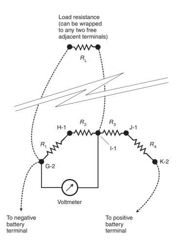
**Figure DC14-4** *Circuit for testing a resistive voltage divider under load. Dashed lines indicate jumpers. This diagram shows the arrangement for measuring variations in*  $E_2$ *as the load resistance*  $R_L$  *is alternately connected and disconnected from the series combination of*  $R_1$  *and*  $R_2$ .
