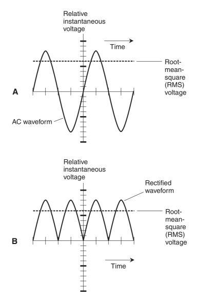
**Figure ACI3-1** Full-wave rectification. At A, the AC waveform as it appears at the power strip. At B, the pulsating DC waveform as it appears at the output of the rectifier. Dashed lines indicate root-mean-square (RMS) or effective voltages.
