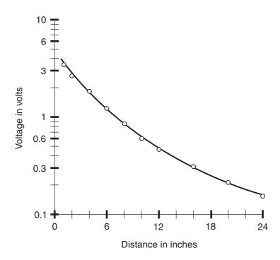
**Figure DC23-2** *Open-circuit voltage from solar module versus distance from miniature lamp. The voltage scale is logarithmic.*
