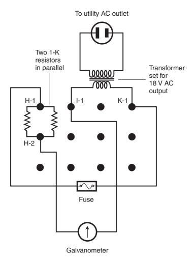
**Figure AC5-2** Suggested breadboard arrangement for testing a galvanometer with AC. The resistors should be rated at 1/2 W, and the transformer should be set for 18 V output. Black dots represent breadboard terminals. Note that when two lines (representing wires) intersect in a circuit diagram without a dot, the wires are not meant to be connected to each other at the point of crossing.
