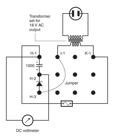
**Figure AC8-1** Addition of a filter capacitor to the half-wave rectifier circuit, and measurement of the open-circuit filtered DC voltage across the capacitor. The value (1000) is stated in microfarads ( $\mu$ F). Pay careful attention to the diode and capacitor polarities! The jumper can serve as a "switch" for the output circuit.
