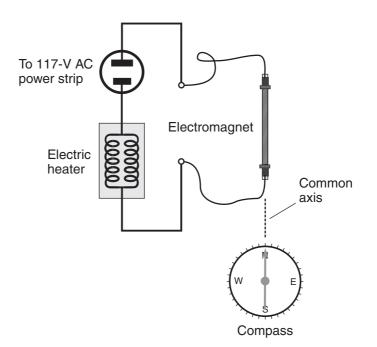
Figure MAG13-2 Compass near the end of an electromagnet. The rod and the compass needle should lie along a common axis with the electromagnet powered-down. What will happen when you supply the coil with AC?
