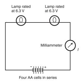
Figure DC18-3 Measurement of current I drawn by the combination of two "identical" lamps in series.
