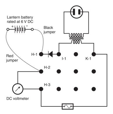
**Figure AC9-2** *Measurement of the open-circuit pulsating DC output voltage from the transformer-diode-battery combination with the battery connected "forward" so its voltage adds to the rectified voltage.*
