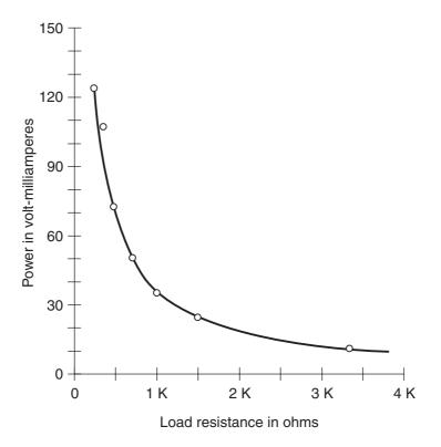
**Figure DC24-3** *Graph of volt-milliampere (VmA) power from solar module versus load resistance in direct sunlight.*
