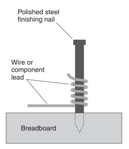
**Figure DC1-2** Wire-wrapping technique. Wind the wire or component lead at least twice, but preferably four or five times, around the nail. Extra wire should be snipped off if necessary, using a diagonal cutter.
