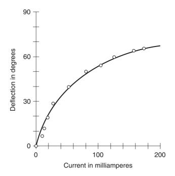
**Figure DC22-4** *Compass needle deflection versus coil current for a DC galvanometer. This graph is based on my experimental results, which appear in Table DC22-1.*
