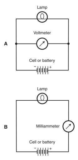
**Figure DC16-1** *At A, the arrangement for measuring the voltage across a lamp. At B, the arrangement for measuring the current through a lamp.*
