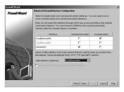
**FIGURE 15.20** Cisco Router and Security Device Manager Advanced Firewall DMZ Service Configuration
