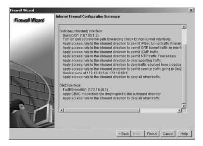
Next, as shown in Figure 15.28, you see the familiar delivery screen. Note the number of commands that are going to be delivered this time. The commands have gone up significantly in number, largely because the office now has a DMZ interface, and this makes the configuration more complex.
