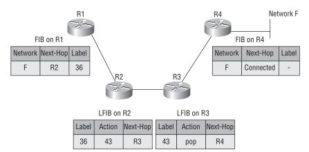
FIGURE 11.17 Forwarding a Packet through MPLS
