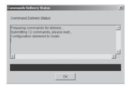
Once the configuration has been delivered to the router, click OK. After the wizard is complete, the Edit IPS tab on the Intrusion Prevention System (IPS) page opens, as shown in Figure 16.14. Make sure that you have the Edit IPS tab selected.
