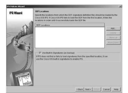
FIGURE 16.9 SDF Locations Screen
