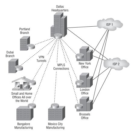
FIGURE 1.4 FutureTech VPN Connections and Physical Plant Locations
