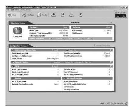
Next, click the Configure button in the main toolbar at the top of the screen. When the Configuration screen (shown in Figure 16.4) opens, the Interface and Connections button in the Tasks bar is selected.
