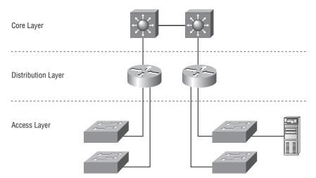
FIGURE 1.1 Three-layer hierarchical design model
