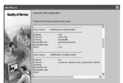
FIGURE 18.14 Signaling and Streaming Video Classes
