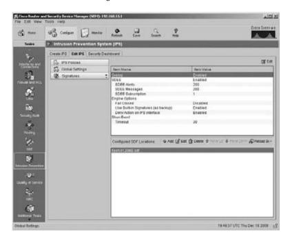
Finally, you can access the last of the three editing features on the Edit tab by clicking the Signatures button. Figure 16.16 shows the Signatures screen. You will most likely spend most of your time in this screen; this is where you can tune, enable, or disable signatures that are in the database. You can filter or look at just a specific group of signatures by selecting a folder from the drop-down list on the left side of the screen.
