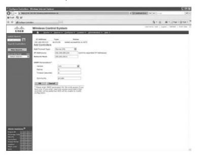
**5.** Go back up to the Configure menu and click Controllers again. When the All Controllers page opens, you will see the WLC that you added. Figure 20.19 shows the All Controllers page with the WLC that I added.
