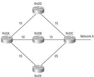
FIGURE 5.6 Unequal-Cost Load Balancing
