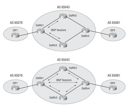
FIGURE 7.3 Partial Mesh vs. Full Mesh
