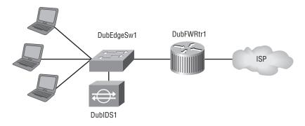
For traffic to reach the sensor, the switch, DubEdgeSw1, must send it there. When the IDS sensor detects malicious traffic, it sends an alert to the local IT monitoring station. Local IT personnel then configure the firewall to block further traffic from that source.
