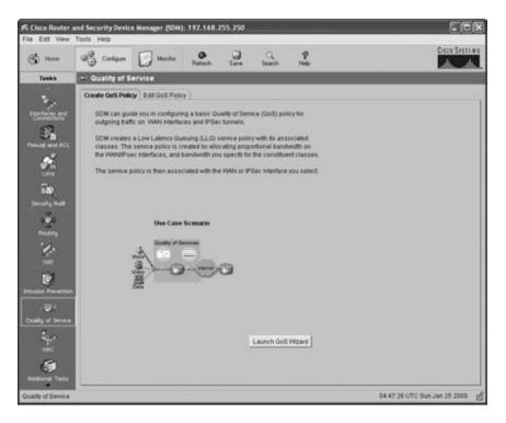
Figure 18.8 shows the opening screen for the QoS Wizard. This wizard is going to guide you through the process of creating a QoS policy for a WAN interface. The SDM will create a policy that handles two main types of traffic. The first is real-time traffic, which handles voice traffic and its signaling traffic. The second is business-critical traffic. The business-critical traffic is broken down into three subcategories:
