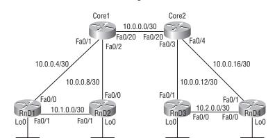
FIGURE 5.4 EIGRP Test Network Configuration
