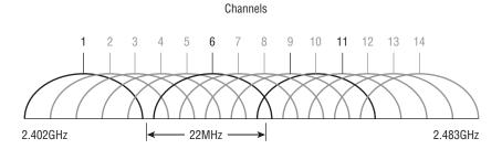
In the U.S.A., only 11 channels are configurable, with channels 1, 6, and 11 being non-overlapping. This allows you to have three access points in the same area without experiencing interference.
