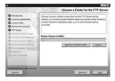
9. Specify the folder to be used for TFTP server files. Again, Cisco recommends that the folder be located on a path different from that of the WCS installation. This preserves files uploaded from or downloaded to controllers should you ever uninstall WCS. The default path, as shown in Figure 20.7, is C:\. Click Choose and specify a different path, one that is appropriate for your system. When you are finished, click Next to continue.
