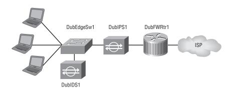
IPS is different from IDS. When the IPS detects malicious traffic, it can also send an alert to the management station. But, more importantly, it can immediately block the malicious traffic. The traffic is blocked by the IPS, not by another device, so the original and
