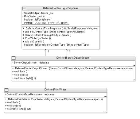
**Figure 6-16.** *Diagram over the* DeferredContentType *implementation*
