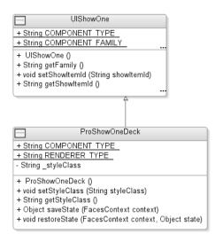
Figure 3-11. Class diagram showing the ProShowOneDeck class
