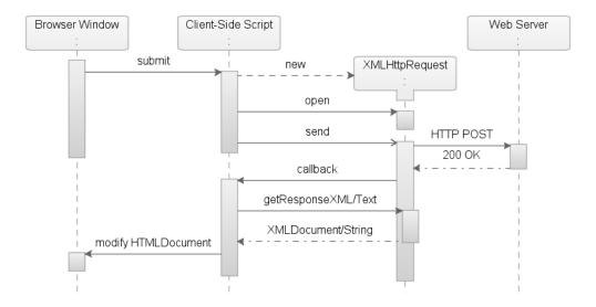
**Figure 4-2.** Sequence diagram over an XMLHttpRequest postback
