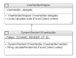
Figure 10-3. Class diagram showing the DynamicRenderKitViewHandler implementation
