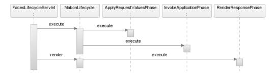
Figure 7-10. Sequence diagram over Mabon lifecycle during postback
