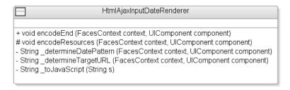
Figure 7-5. Class diagram showing the HtmlAjaxInputDateRenderer
