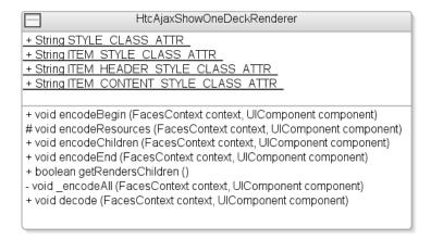
**Figure 9-10.** Class diagram showing the HtcAjaxShowOneDeckRenderer class
