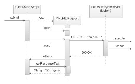
Figure 7-9. Sequence diagram of Mabon/Ajax data fetch request
