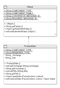
Figure 2-10. Class diagram over the ProInputDate renderer-specific subclass
