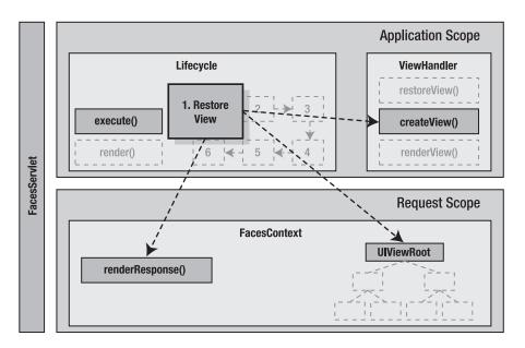
Figure 1-11. Restore View phase during initial request
