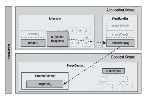
Figure 1-12. Render Response phase during initial request
