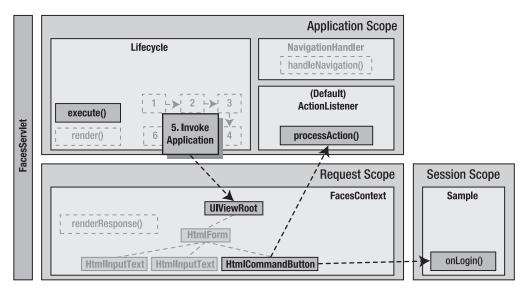
Figure 1-21. Performing application logic
