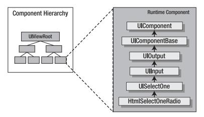
Figure 1-7. UIComponent inheritance
