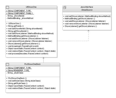
**Figure 3-8.** Class diagram showing the UIShowOne implementation
