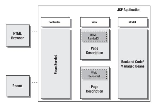
**Figure 1-3.** *MVC architecture with JSF (Model 2)*
