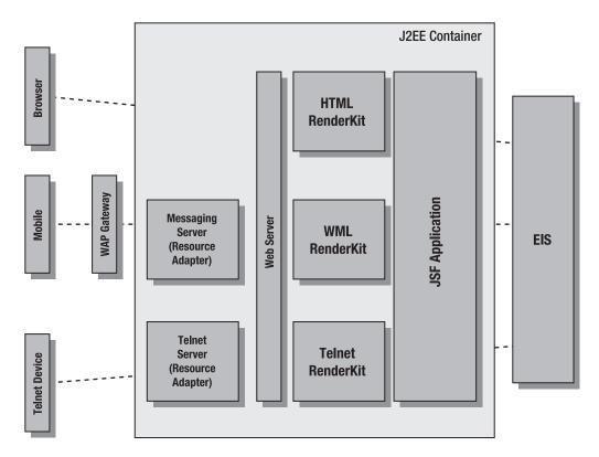
**Figure 1-2.** J2EE architecture using JSF for a typical multitier software solution, serving a retail company
