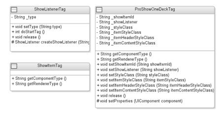
**Figure 3-12.** Class diagram showing the three tag handlers
