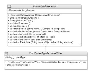
Figure 6-10. Diagram of FixedContentTypeResponseWriter
