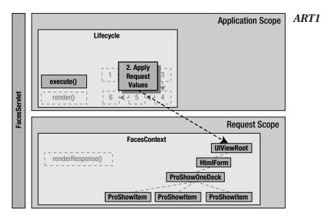
**Figure 3-6.** Event handling in the Apply Request Values phase
