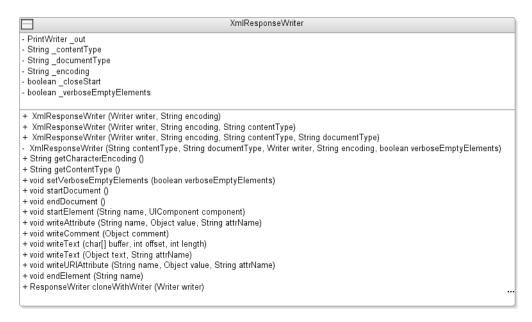
Figure 8-15. Class diagram showing the XMLResponseWriter class
