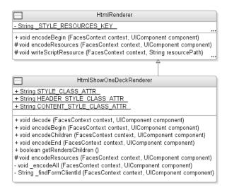
Figure 3-10. Class diagram showing the HtmlShowOneDeckRenderer extending the HtmlRenderer
