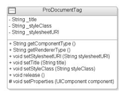
Figure 8-12. Class diagram showing the ProDocumentTag class
