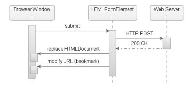
Figure 4-1. Sequence diagram over a regular postback
