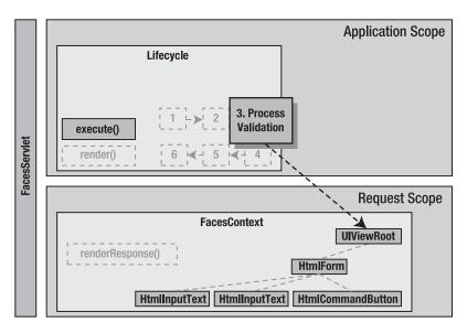
Figure 1-19. Performing conversion and validation
