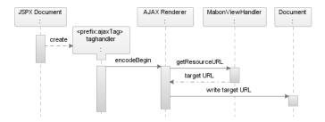
Figure 7-8. Sequence diagram of Mabon initial request
