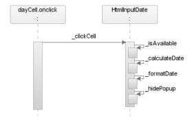
Figure 7-13. HtmlInputDate.prototype. clickCell method
