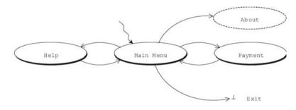
*Figure 10.6 The Park applet's GUI structure*
