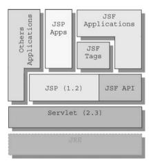
Figure 9.11 Basic technology stack for server-side Java Web GUIs
