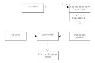
Figure 6.14 The Command design pattern
