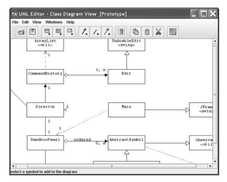
Figure 3.6 A UML class diagram editor
