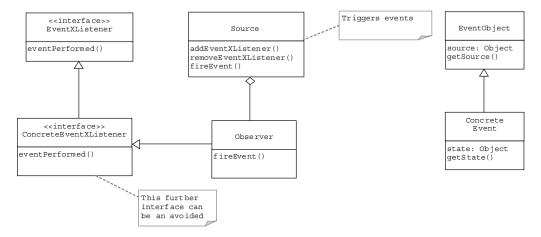
Figure 6.6 shows the classes involved in this approach. Compare this with Figure 6.4, which shows the classic Observer pattern.
