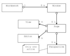
Figure 13.5 Eclipse workbench structure
