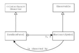
Figure 16.8 Making objects communicate with their container
