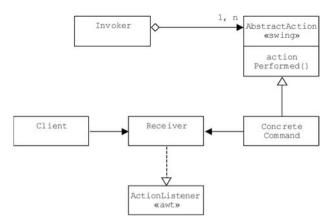
Figure 16.14 The Command design pattern
