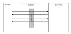
*Figure 9.3 Web application with thin control*
