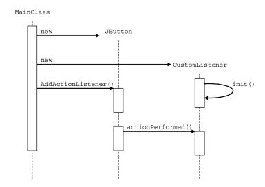
Figure 1.9 A sample sequence diagram
