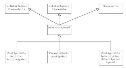
*Figure 14.18 Class diagram for the local container's symbols*
