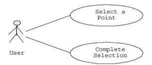
*Figure 3.8* The use case diagram for a geographic point chooser component
