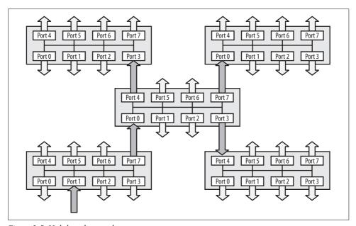
Figure 2-5. Hub-based network
