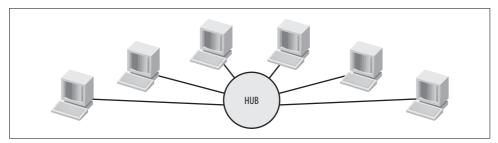
Figure 2-2. Hub connecting multiple hosts to a network
