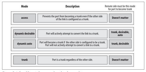
Figure 5-4. Possible switch port modes related to trunking
