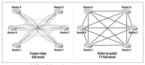
Figure 22-7. Six-node fully meshed networks
