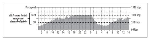
Figure 22-4. Frame-relay CIR and DE frames
