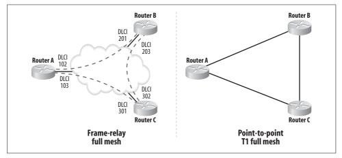
Figure 22-6. Frame-relay versus point-to-point T1 meshed networks
