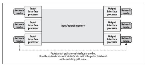
Figure 15-1. Router switching requirements
