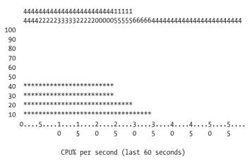
The router was running at an average of 4 percent CPU utilization with CEF running. When I disabled all route caching, the router reverted to process switching for all packets. For just 600k of traffic, the router is now using 40 percent of its CPU cycles to forward the packets.
