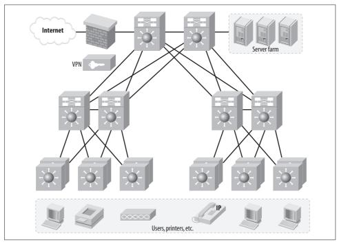
Figure 33-9. Typical three-tiered corporate network
