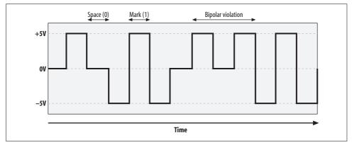
Figure 20-2. T1 AMI signaling
