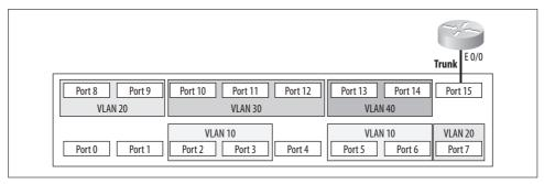
Figure 4-5. Router on a stick
