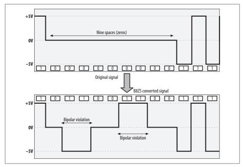
Figure 20-3. B8ZS zero substitution
