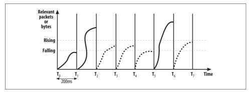
Figure 18-3. Rising and falling thresholds
