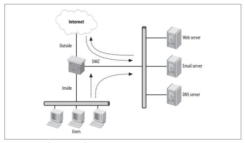
Figure 25-1. Simple DMZ network
