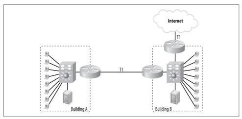
Figure 29-4. Simple two-building VoIP network
