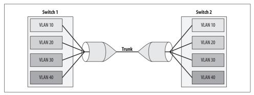
Figure 5-2. Visual representation of a trunk
