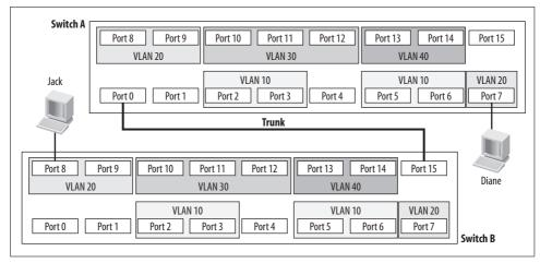
Figure 4-3. Two switches connected with a trunk
