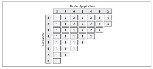
Figure 7-3. EtherChannel physical link balancing
