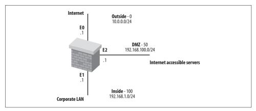
Figure 26-5. Firewall with DMZ
