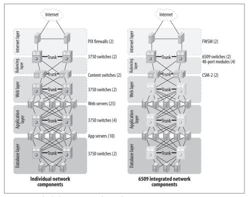
Figure 17-1. Individual versus integrated network components
