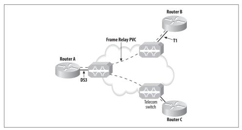
Figure 22-1. Simple frame-relay WAN
