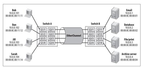
Figure 7-4. EtherChannel load-balancing factors
