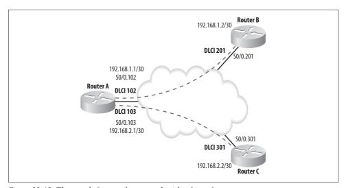
Figure 22-12. Three-node frame-relay network with subinterfaces
