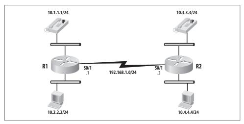
Figure 32-1. Simple converged network
