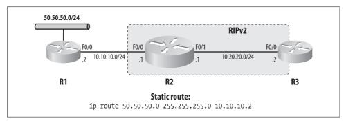
Figure 11-2. Redistributing a static route into RIPv2
