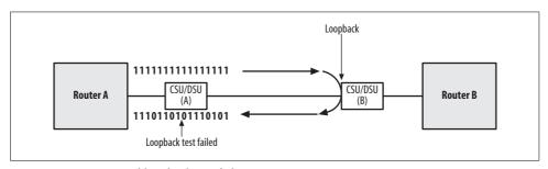
Figure 20-9. Conceptual loopback test failure
