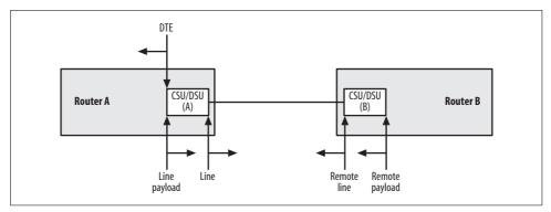
Figure 20-13. Integrated CSU/DSU loopback points
