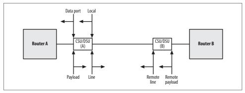
Figure 20-11. Loopback points in CSU/DSUs
