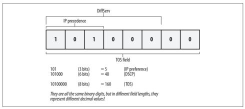
Figure 29-6. Different decimal values depending on the number of significant bits in the TOS field
