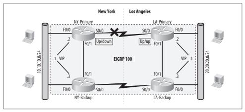
Figure 13-6. Better failover design using EIGRP
