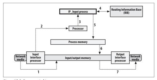
Figure 15-2. Process switching
