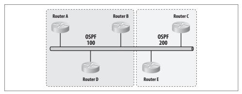
Figure 10-2. Two OSPF processes on a single network
