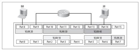
Figure 4-2. External routing between VLANs
