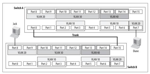
Figure 5-1. A trunk connecting two switches
