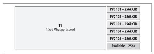
Figure 22-8. Subscription of a T1 using frame-relay PVCs
