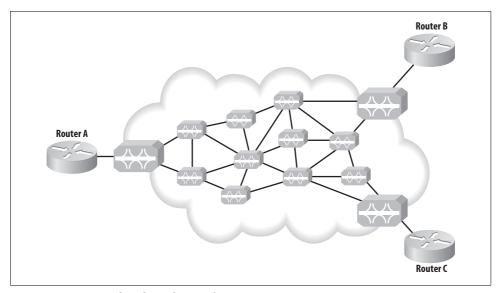
Figure 22-2. Frame-relay physical network
