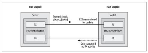
Figure 3-3. Common auto-negotiation failure scenario
