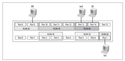
Figure 4-1. VLANs on a switch
