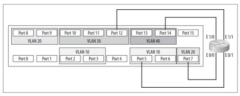
Figure 4-4. Routing between multiple VLANs
