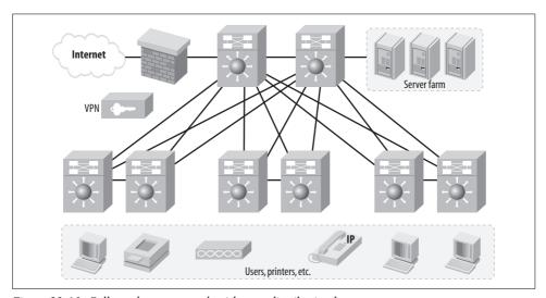
Figure 33-10. Collapsed-core network without a distribution layer
