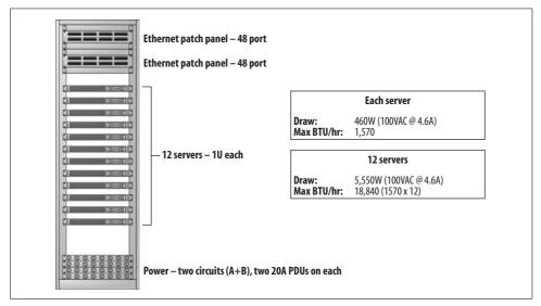
Figure 33-8. Figuring out how many servers can fit in a rack
