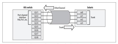
Figure 7-2. Cisco and Solaris terminology regarding EtherChannels
