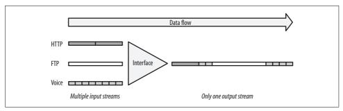
Figure 29-3. Packets through a serial interface
