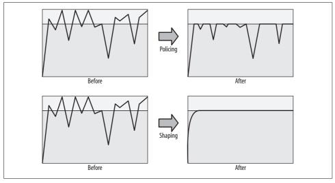
Figure 29-7. Traffic policing versus traffic shaping
