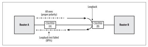
Figure 20-10. BPVs seen during loopback test
