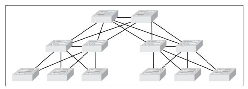
Figure 6-1. Three-tier switched network
