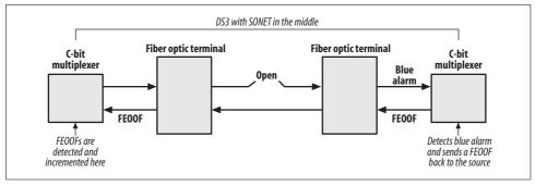
Figure 21-3. Far-end out-of-frame errors
