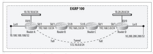
Figure 12-2. Simple network with a tunnel
