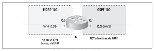
Figure 11-1. Most routing protocols do not redistribute by default
