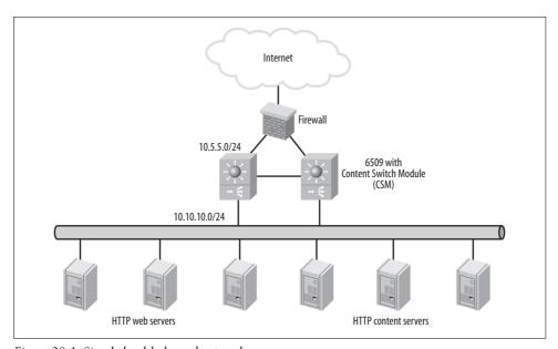
Figure 28-1. Simple load-balanced network
