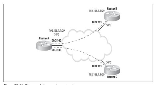
Figure 22-11. Three-node frame-relay network
