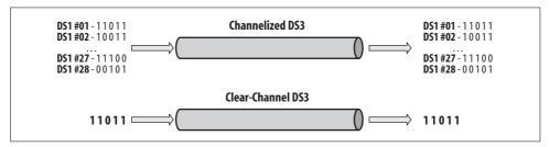
Figure 21-4. Channelized versus clear-channel DS3
