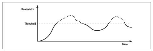
Figure 18-1. Incorrect storm-control model
