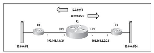
*Figure* 9-1. *Same network with different prefix lengths*
