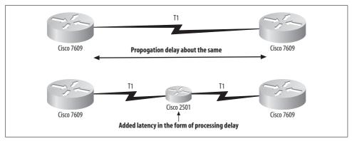
Figure 19-5. Processing delay
