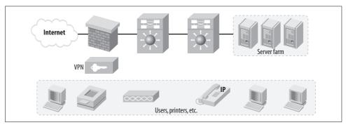
Figure 33-11. Collapsed-core network consisting of only one layer
