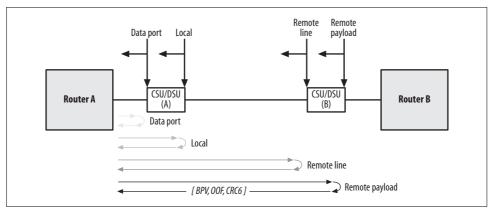
Figure 20-12. Loopback testing progression
