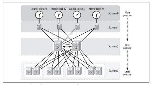
Figure 35-2. NTP hierarchy in a corporate network
