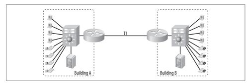
Figure 30-1. Two-building network with a single T1
