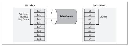
Figure 7-1. EtherChannel on IOS and CatOS
