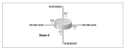
Figure 10-10. Routing protocol network interfaces
