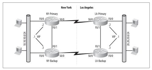
Figure 13-4. Two-link failover scenario using HSRP
