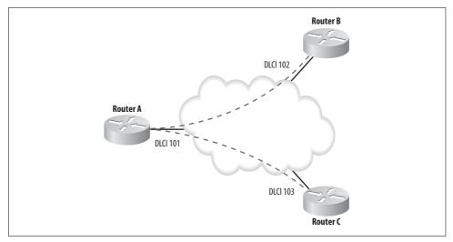
Figure 22-3. DLCIs in a frame-relay network
