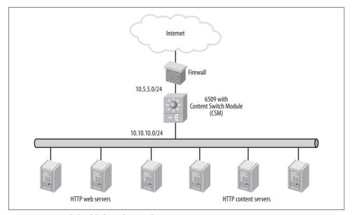
Figure 27-1. Simple load-balanced network
