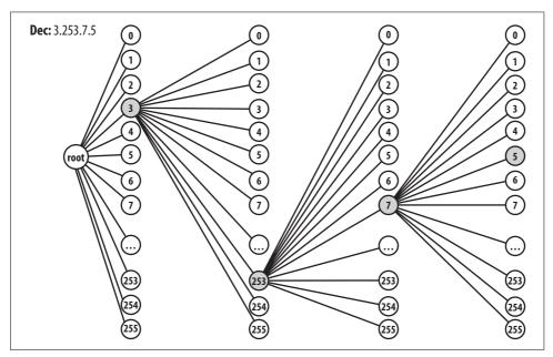
Figure 15-5. Optimum-switching multiway tree
