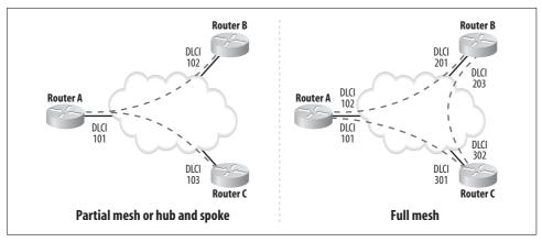
Figure 22-5. Meshed frame-relay networks
