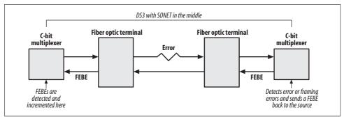
Figure 21-2. Far-end block errors
