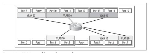
Figure 16-1. VLANs routed from within a switch
