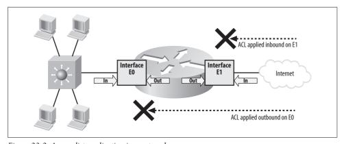
Figure 23-2. Access-list application in a network
