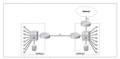
Figure 29-1. Simple two-building network
