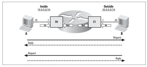
Figure 23-3. Simple network without ACLs
