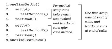
Figure 3.2: Execution Order of Setup Code
