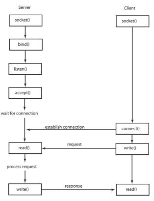
Figure 21.1 TCP connection protocol.
