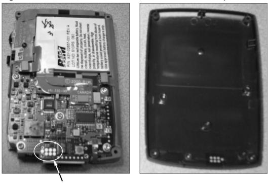
Figure 14.4 External Interface on Research In Motion's BlackBerry 957 Device
