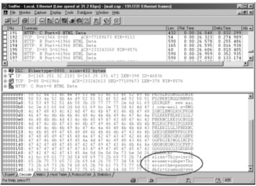
Figure 10.4 Sniffer Pro Displaying Captured Data
