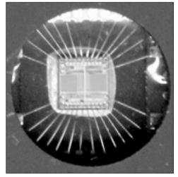
**Figure 14.11** Magnified Portion of a ROM Die Showing Actual Data Bits Photo courtesy of ADSR Ltd., www.adsr.de
