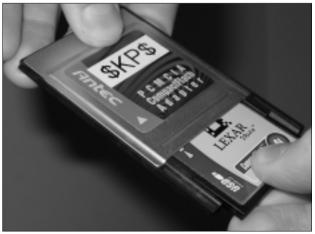
CompactFlash cards are compatible with the ATA/IDE hard drive specification, so most operating systems will automatically detect the cards without the need for additional drivers. The card was automatically detected by a laptop running OpenBSD 3.0:
