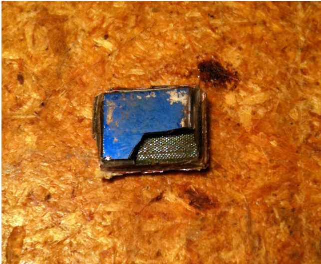
A piece of the processor chip came off.
