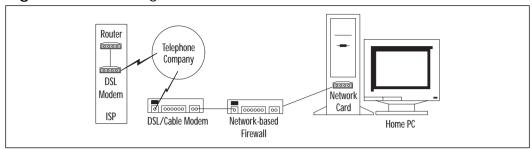
Figure 8.32 Installing the Siemens External DSL/Cable Router
