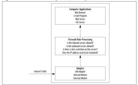
Figure 5.15 Firewall Processing Conceptual Diagram
