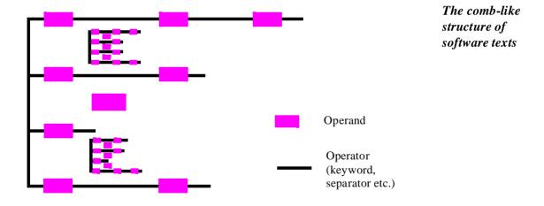
Each branch of the comb is a sequence of alternating operators and operands; it should normally begin and end with an operator. In the space between two branches you find either a single operand or, recursively, a similar comb-like structure.
