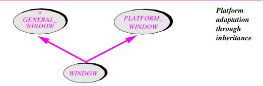
Class *GENERAL\_WINDOW* and similar ones such as *GENERAL\_BUTTON* are deferred: they express all that can be said about the corresponding graphical objects and the applicable operations without reference to a particular graphical platform. Classes such as *PLATFORM\_WINDOW* provide the link to a graphical platform such as Windows, OS/2-Presentation-Manager or Unix-Motif; they give access to the platform-specific mechanisms (encapsulated through a library such as WEL or MEL).
