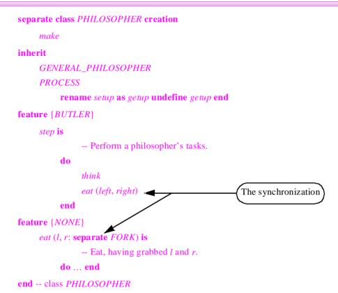
The entire synchronization requirement is embodied by the call to *eat*, which uses arguments *left* and *right* representing the two necessary forks, thus reserving these objects.
