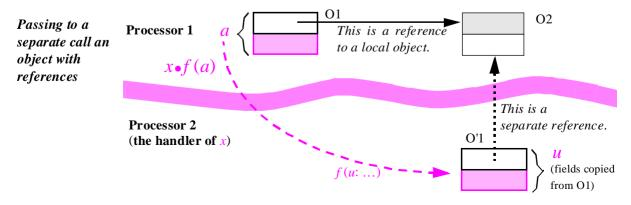
The figure illustrates the case in which the formal argument u is itself expanded. Then the attachment is simply a copy of the fields of the object O1 onto those of the object O'1 attached to u. Permitting O1 to contain a reference would produce a traitor field in O'1. The problem would also arise if O1 had a subobject with a reference; hence the mention "directly or indirectly" in the rule.
