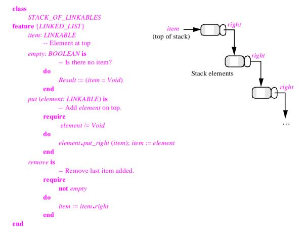
The stack representation, as pictured, takes advantage of the *right* field already present in every *LINKABLE* to link all recycled elements without using any extra space. *LINKABLE* must export *right* and *put\_right* to *STACK\_OF\_LINKABLES* as well as *LINKED\_LIST*.
