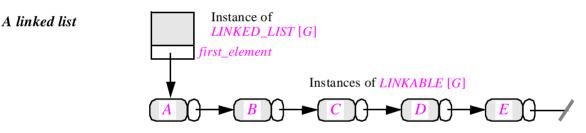
This representation makes insertion or deletion fast if you have a reference to the linkable immediately to the left of the operation's target: a few reference manipulations will do, as shown here for the deletion of the third element.
