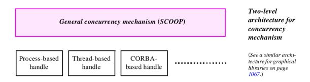
At the highest level the mechanism is platform-independent. This is the level which most applications use, and which this chapter describes. To perform concurrent computation, applications simply use the **separate** mechanism.
