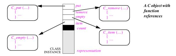
For example, a C structure type *REAL\_STACK* may be declared by the type definition
