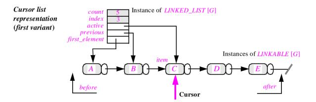
Along with *first\_element* it will be useful to keep two references in the list header, enabling us to perform insertions and deletions efficiently: *active*, attached to the cursor item at cursor position, and *previous* attached to the previous one.
