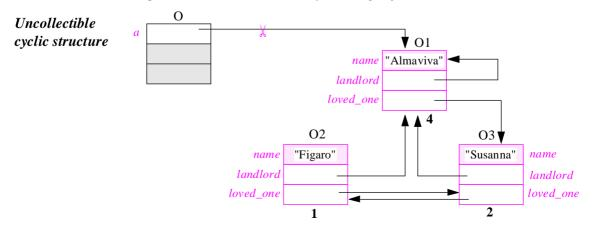
The objects in the right part of the figure, O1, O2 and O3, contain cyclic references to each other; assume that no outside object other than O contains a reference to any of these objects. The corresponding reference counts have been displayed below each object.
