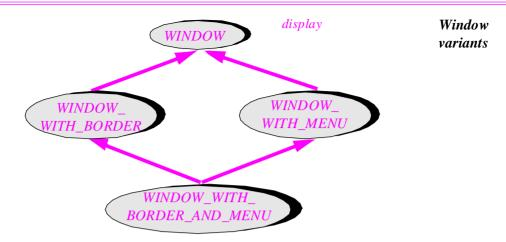
In class *WINDOW\_WITH\_BORDER\_AND\_MENU* we will again redefine *display*; here the redefined version should apply the standard window display, then display the border, then display the menu.
