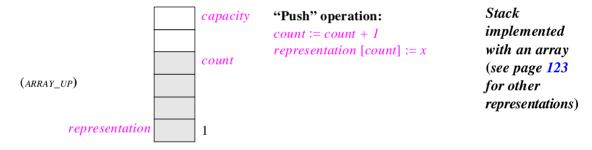
The array will be called *representation* and will have bounds 1 and *capacity*; the implementation also uses an integer, the attribute *count*, to mark the top of the stack.
