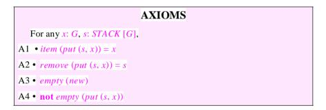
The first two axioms express the basic LIFO (last-in, first-out) property of stacks. To understand them, assume we have a stack *s* and an instance *x*, and define *s'* to be *put* (*s*, *x*), that is to say the result of pushing *x* onto *s*. Adapting an earlier figure:
