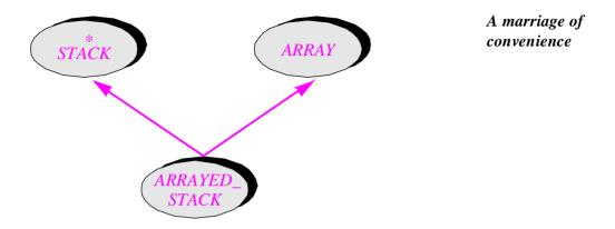
Consider the implementation of stacks as arrays. Since classes are available to cover stacks as well as arrays (deferred for *STACK*, effective for *ARRAY*, both seen in earlier chapters), the best way to implement class *ARRAYED\_STACK*, describing stacks implemented as arrays, is to define it as an heir to both *STACK* and *ARRAY*. This is conceptually right: an arrayed stack is a stack (as seen by clients) and is also an array (internally). The general form is:
