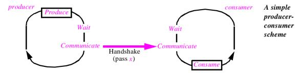
Communication occurs when both processes are ready for each other; this is sometimes called a *handshake* or *rendez-vous*. The design of synchronization mechanisms — enabling us in particular to express precisely the instructions to "Make it known that *process* is ready" and "Wait for *process* to be ready" — has been a fertile area of research and development for several decades.
