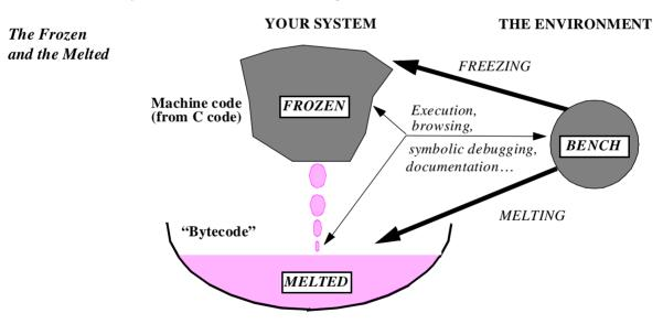
The tricky part (for the compiler implementers) is of course to make sure that the various components can work together, in particular that frozen code can call melted elements — even though it was not known, at freezing time, that they would later be melted! But the result is definitely worthwhile:
