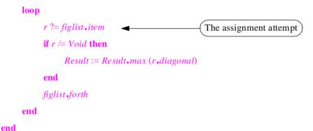
This routine uses the usual iteration mechanisms on sequential structures: *start* to position the traversal on the first element if any, *after* to determine whether there is any element left to examine, *forth* to advance by one position, *item* (defined if **not** *after*) to yield the element at the current cursor position.
