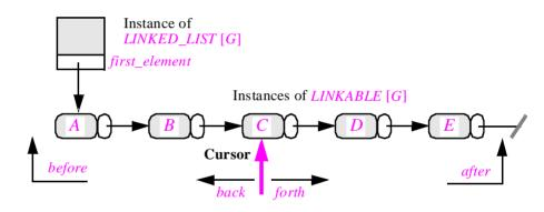
We permit the cursor to be on a list element (if any), or one position to the left of the first, in which case the boolean query *before* will return true, or one position to the right of the last, making *after* true.
