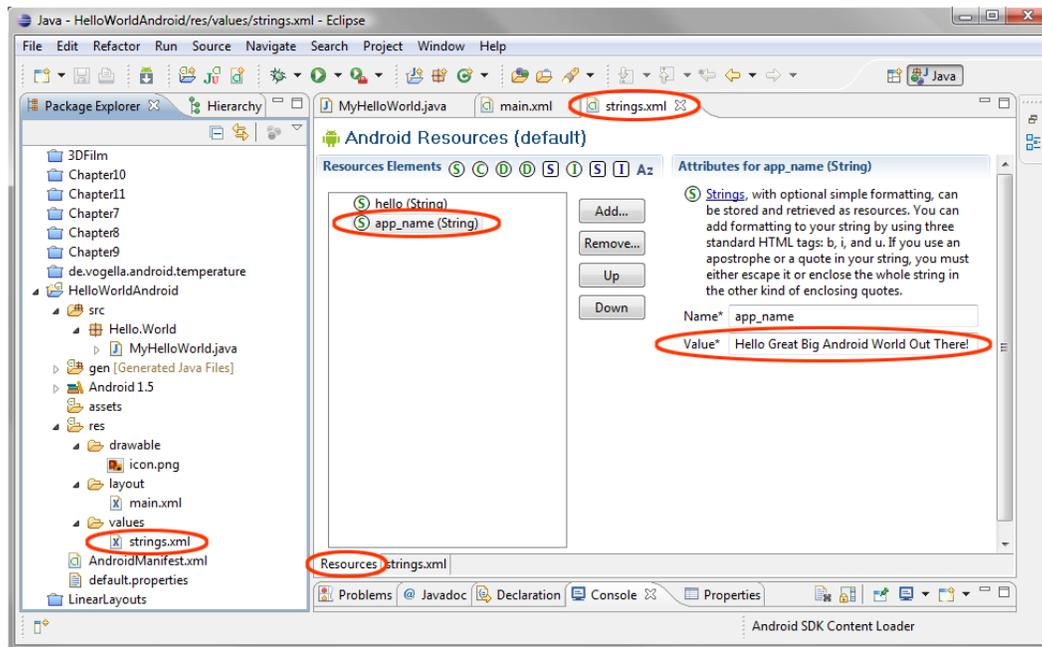
**Figure 4–10.** The `strings.xml` file when it first opens
