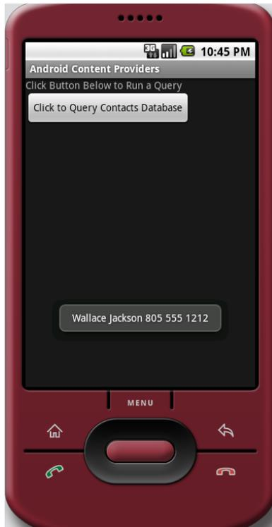
**Figure 10–13.** Running a query in the Android 1.5 emulator
