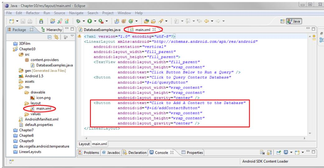
**Figure 10–14.** Adding our second button in main.xml
