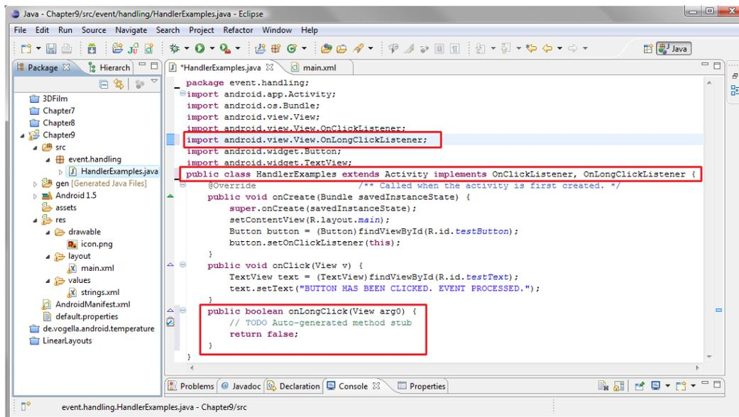
**Figure 9–10.** Implementing an `OnLongClick` listener in *HandlerExamples.java*
