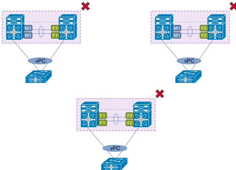
It is not possible to mix different port type inside the same vPC peer-link side (for example bundling M1 port and F1 port on same side of the vPC peer-link) because each port type have different hardware characteristics (in terms of forwarding, queuing, and security).
