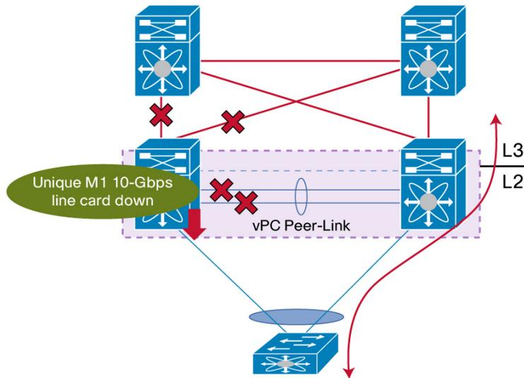
The vPC Object Tracking feature suspends the vPCs on the impaired device so that traffic can be diverted over the remaining vPC peer.
