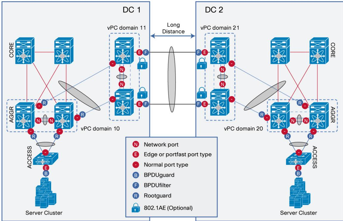
Another design is to interconnect directly between vPC aggregation layer, without using any dedicated vPC layer for DCI. This design is referred to as dual Layer 2 /Layer 3 pod interconnect and is shown in Figure 8.
