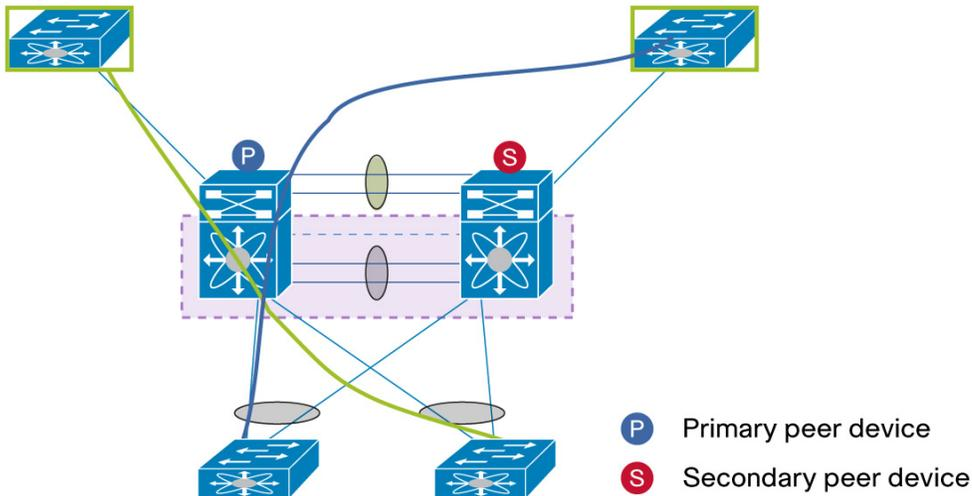
Finally, if you don't want to use non-vPC VLAN to connect the access device to vPC domain (and don't want to create additional inter-switch link between the 2 peer devices), then you can connect the access device to primary peer device using vPC VLAN and leveraging vPC peer-link (Figure 36).
