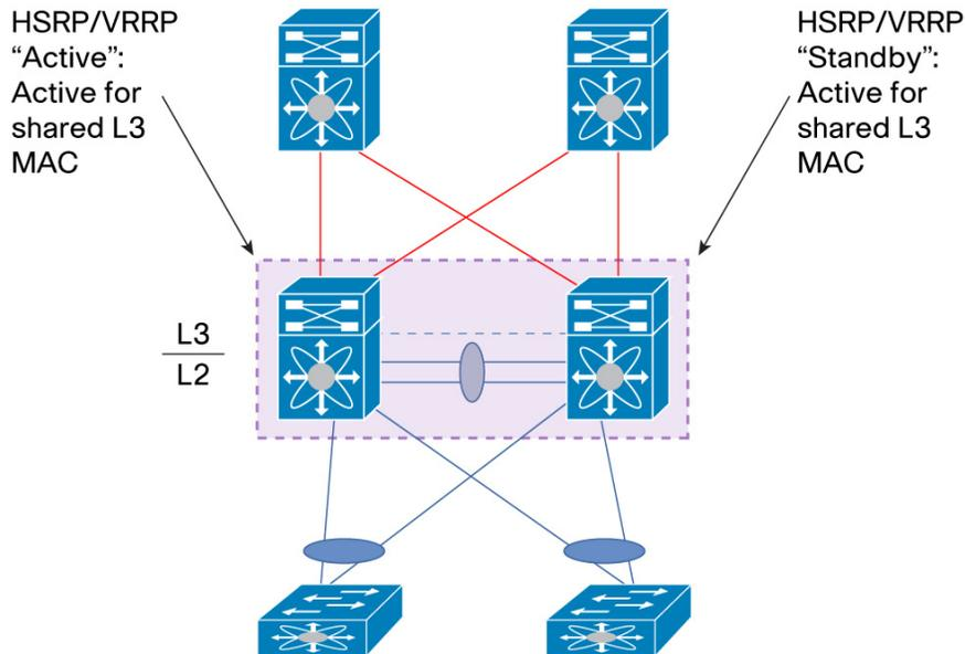
Looking at the show hsrp group command, one vPC peer device appear as the active instance while the other vPC peer device appear as the standby instance. This is the HSRP/VRRP control plane information.
