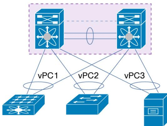
The access device can be any endpoint equipment (L2 switch, rack-mount server, blade server, firewall, load balancer, network attached storage [NAS] device). Only prerequisite for the access device is to support port-channeling (or link aggregation) technology:
