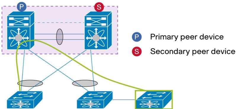
If you can't use an intermediate vPC-attached switch or VDC, the next best alternative is to connect the device to vPC peer devices using a non-vPC VLAN (by definition, a non-vPC VLAN is a VLAN that is not part of any vPC and then not present on vPC peer-link) and create a dedicated inter-switch port-channel to carry these non-vPC VLAN (figure 35).
