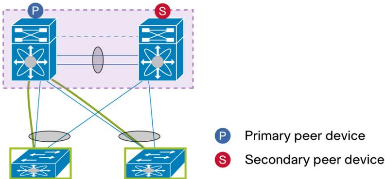
Dual-attaching access device to vPC domain using port-channel provide the following benefits:
