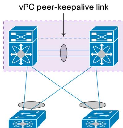
The vPC peer-keepalive link carries periodic heartbeat between vPC peer devices. It is used at the boot up of the vPC systems to guarantee both peer devices are up before forming vPC domain and also when vPC peer-link fails to down state; in the latter case, vPC peer-keepalive link is leveraged to detect split brain scenario (both vPC peer devices are active-active) [when vPC peer-link is down, there is no more real time synchronization between the 2
