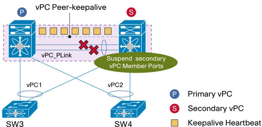
vPC also adds the concept of operationa role: operational primary and operational secondary.
