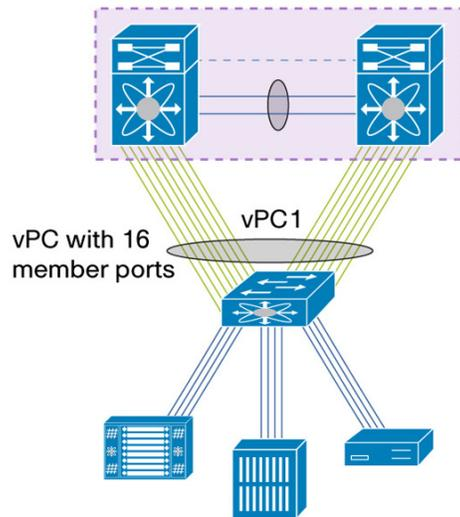
Note: Although not displayed in Figure 4 or 5, orphan ports or active/standby attached devices (that is, using Spanning Tree Protocol) are fully supported in a vPC topology.
