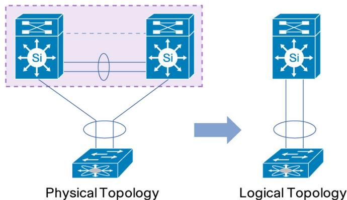
vPC leverages both hardware and software redundancy aspects:
