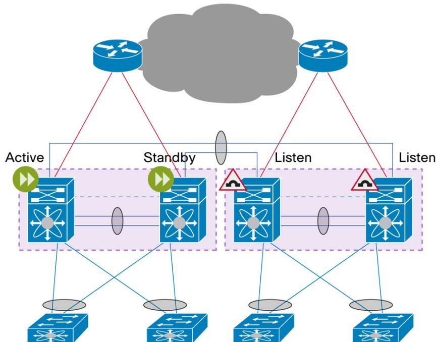
vPC as DCI technology is intended to interconnect two data centers in maximum. If you need to interconnect more than 2 data centers, recommendation is to use Overlay Transport Virtualization (OTV) solution.
