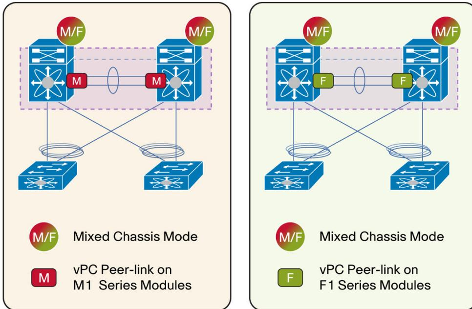
vPC system in mixed chassis mode with peer-link on F1 ports present the following characteristics:
