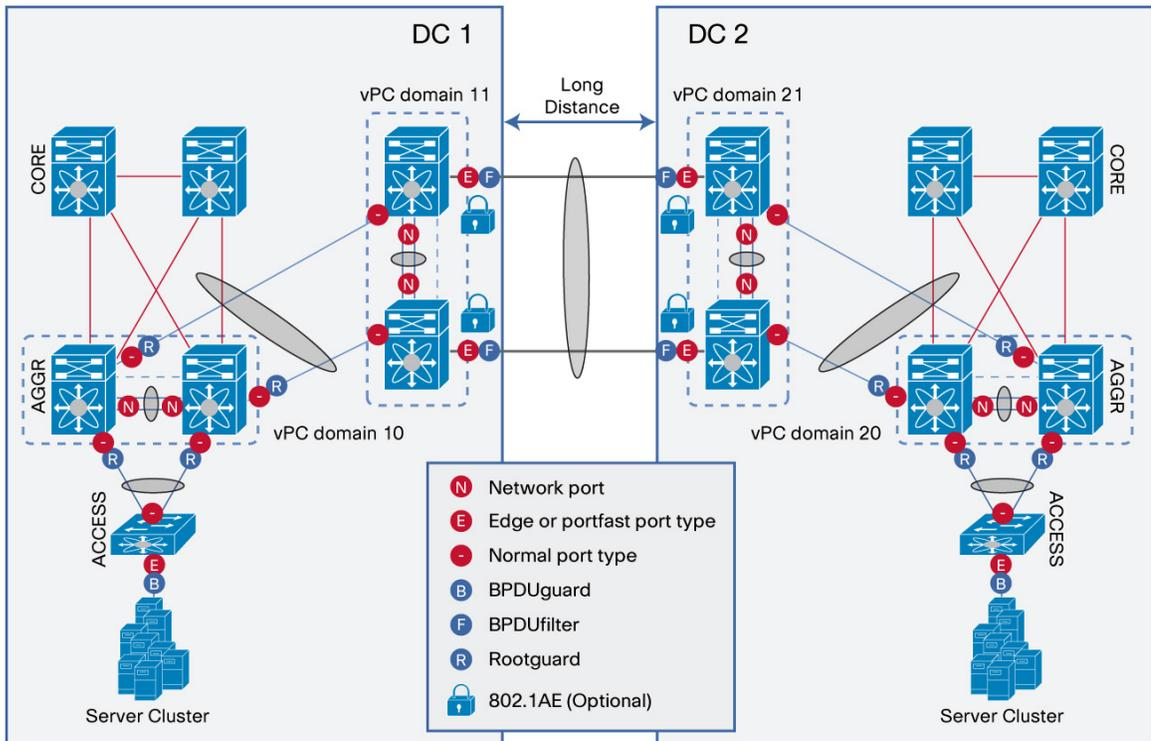
To build successfully a Multilayer vPC for aggregation and DCI solution, use the following guidelines/best practices.
