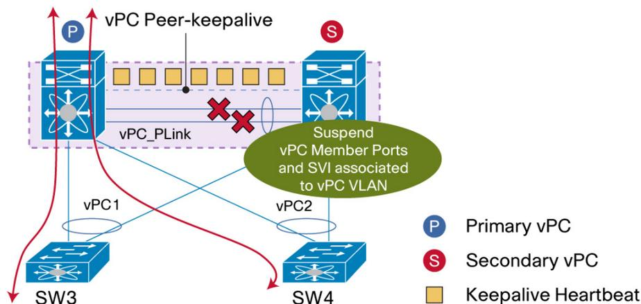
If orphan ports are connected to vPC secondary peer device, they become isolated once peer-link is down. In a VXLAN + vPC implementation, when a vPC peer-link shuts down, all Layer 2 or Layer 3 orphan receivers behind the non-forwarder (shut down vPC peer-link) will not receive any traffic.
