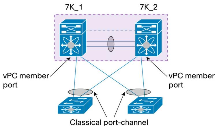
Note: The Layer 3 port-channel is not supported with vPC technology.
