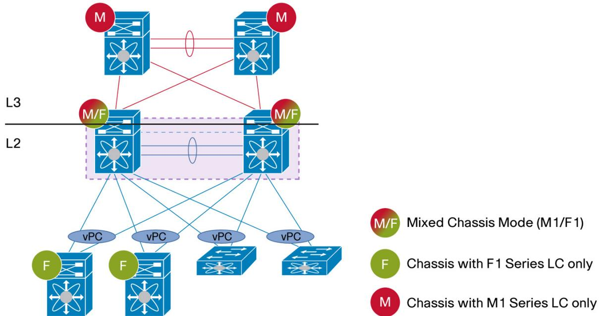
2 different topologies can be implemented with vPC in mixed chassis mode, depending on the nature of vPC peer-link: peer-link on M1 ports and peer-link on F1 ports.
