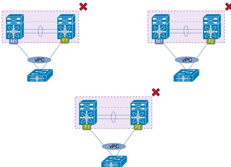
Note: M132XP and M108X2 (32 10-Gigabit Ethernet line cards and 8 10-Gigabit Ethernet line cards, respectively) can form a port-channel together and then can co-exist in the same vPC member port. However, be aware of the requirement that ports on M132XP can form a port-channel or vPC member port with ports on M108X2 only if M132XP ports are configured in dedicated mode.
