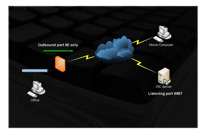
Imagine you are at the office, which is protected by a firewall with strict outbound rules, allowing only outbound traffic on port 80 (no content inspection). You are an IRC addict and must constantly be connected to your favorite IRC server in order maintain your mental health.
